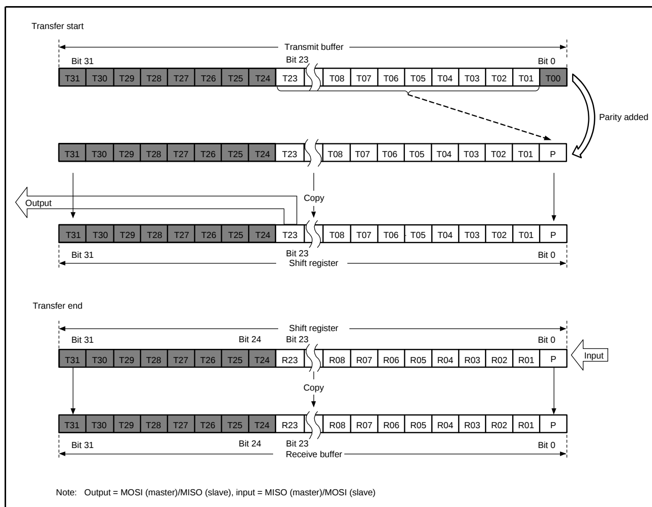
Figure 38.19 MSB First Transfer (24-Bit Data, Parity Enabled)
