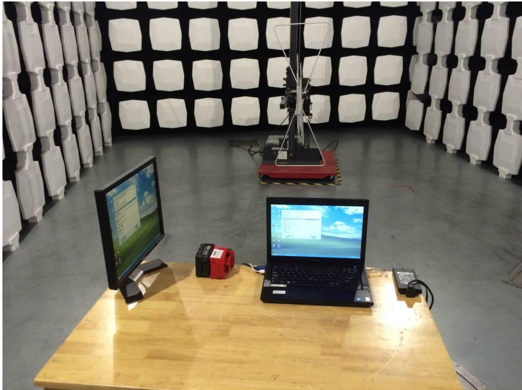
Figure 6 Radiated Emission test setup below 1 GHz
