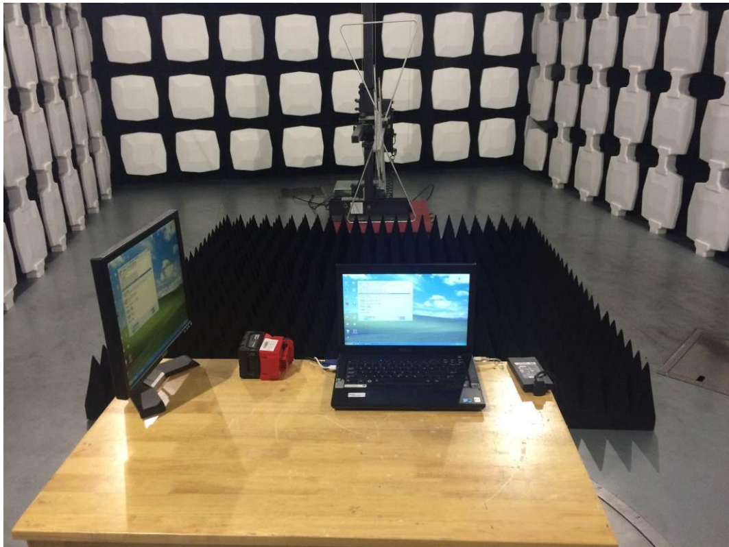
Figure 7 Radiated Emission test setup above 1 GHz
