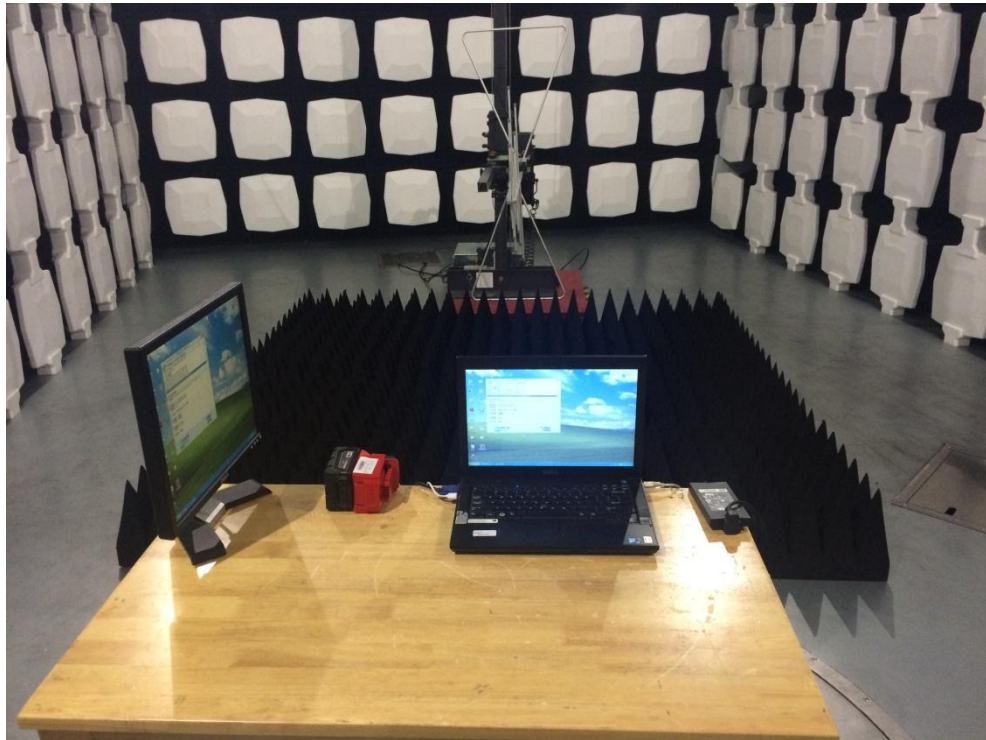
Radiated Emission test setup above 1 GHz
