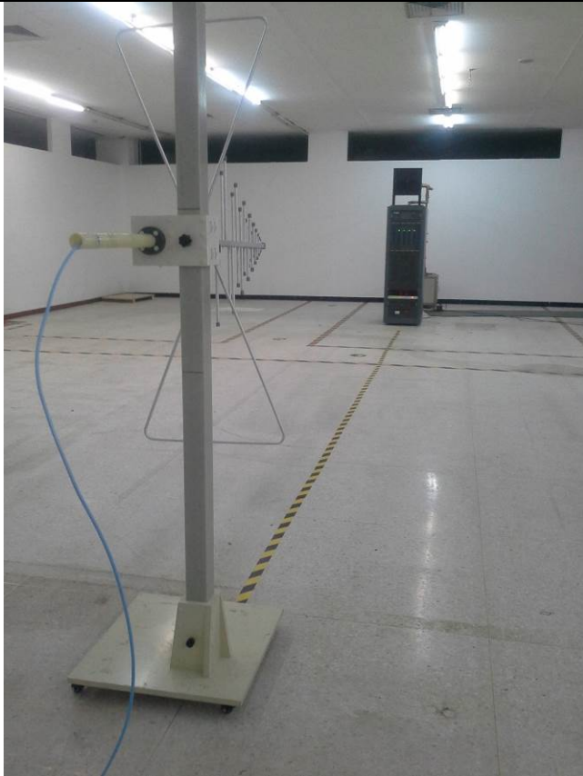
Radiated Spurious Emissions Test Setup Below 1GHz
