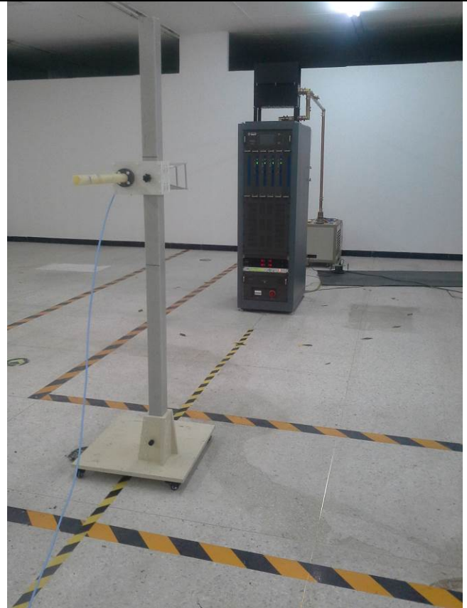
Radiated Spurious Emissions Test Setup Above 1GHz
