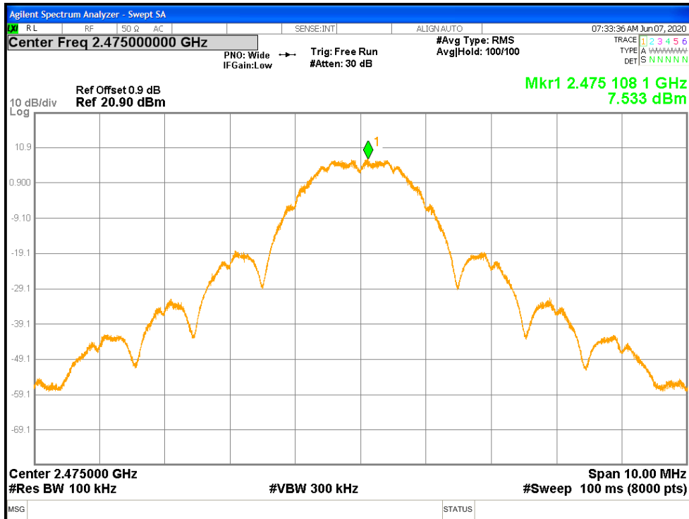
Figure 14: Zigbee Maximum Power Spectral Density-2475 MHz
