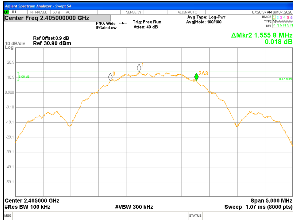
Figure 6: DTS Bandwidth-Transmitter -2405 MHz
