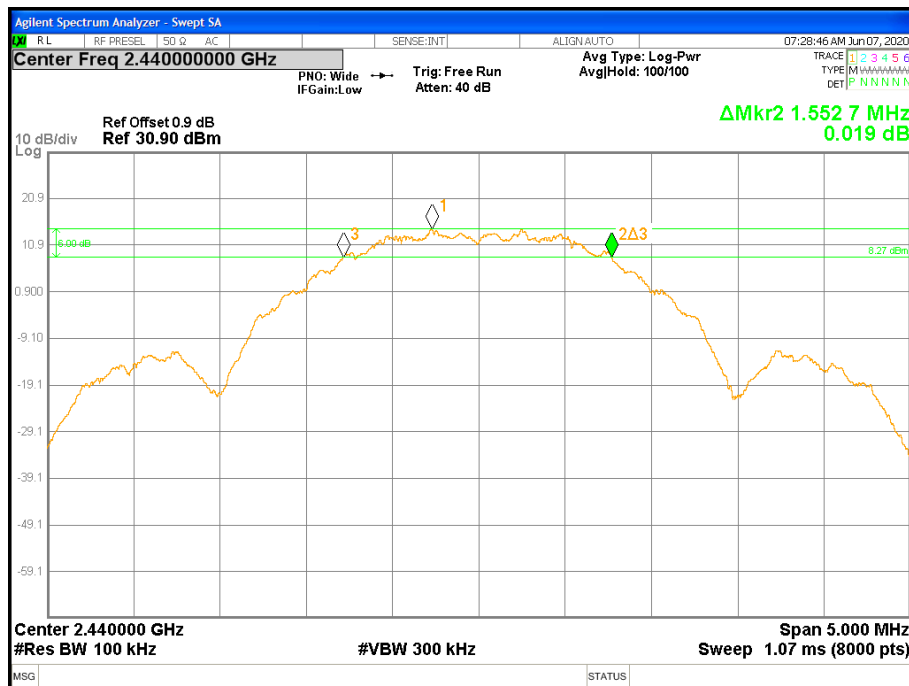
Figure 7: DTS Bandwidth-Transmitter -2440 MHz
