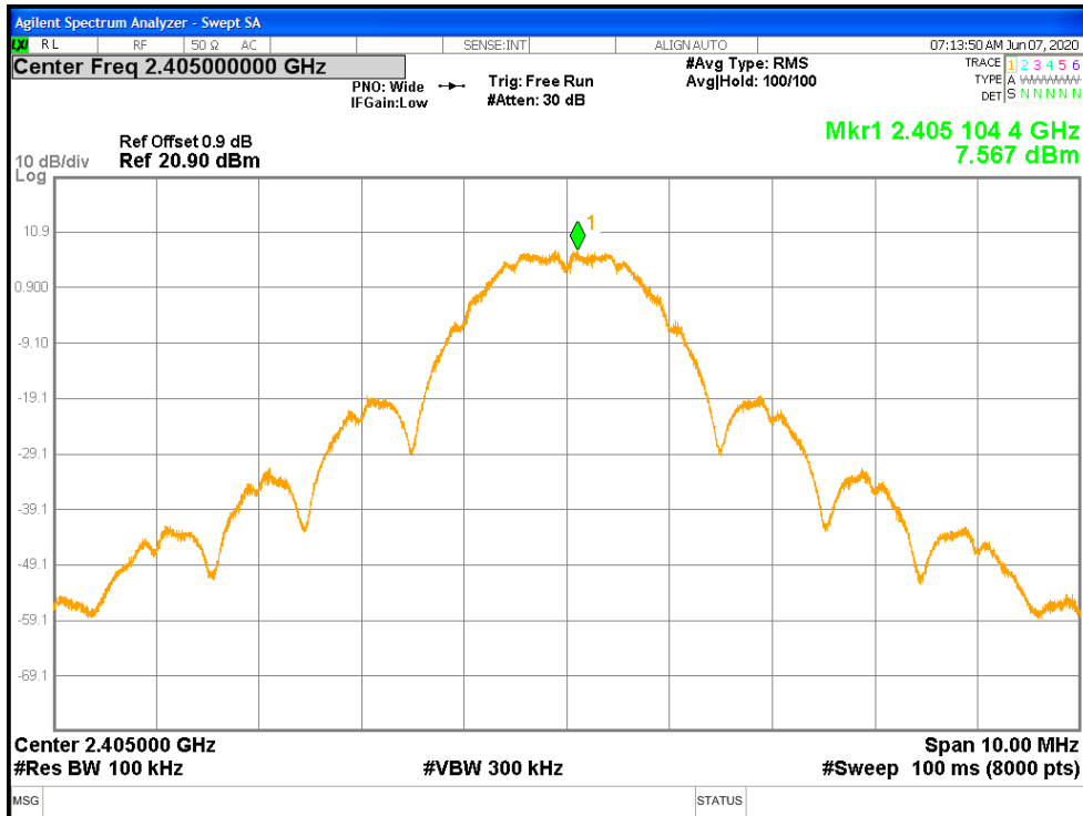
Figure 12: Zigbee Maximum Power Spectral Density-2405 MHz
