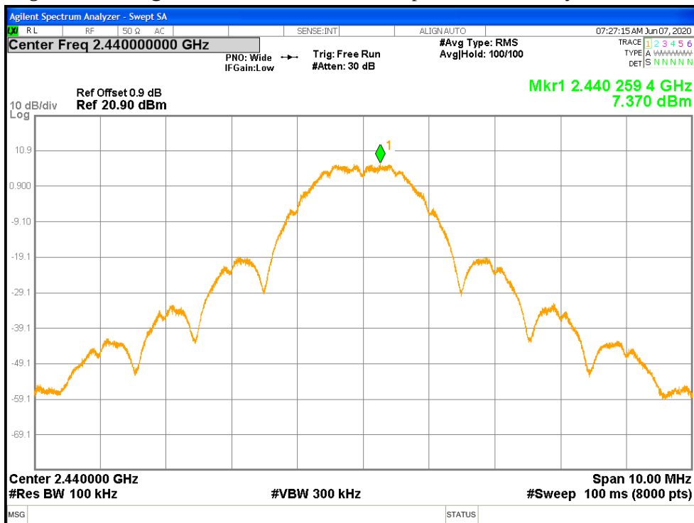
Figure 13: Zigbee Maximum Power Spectral Density-2440 MHz
