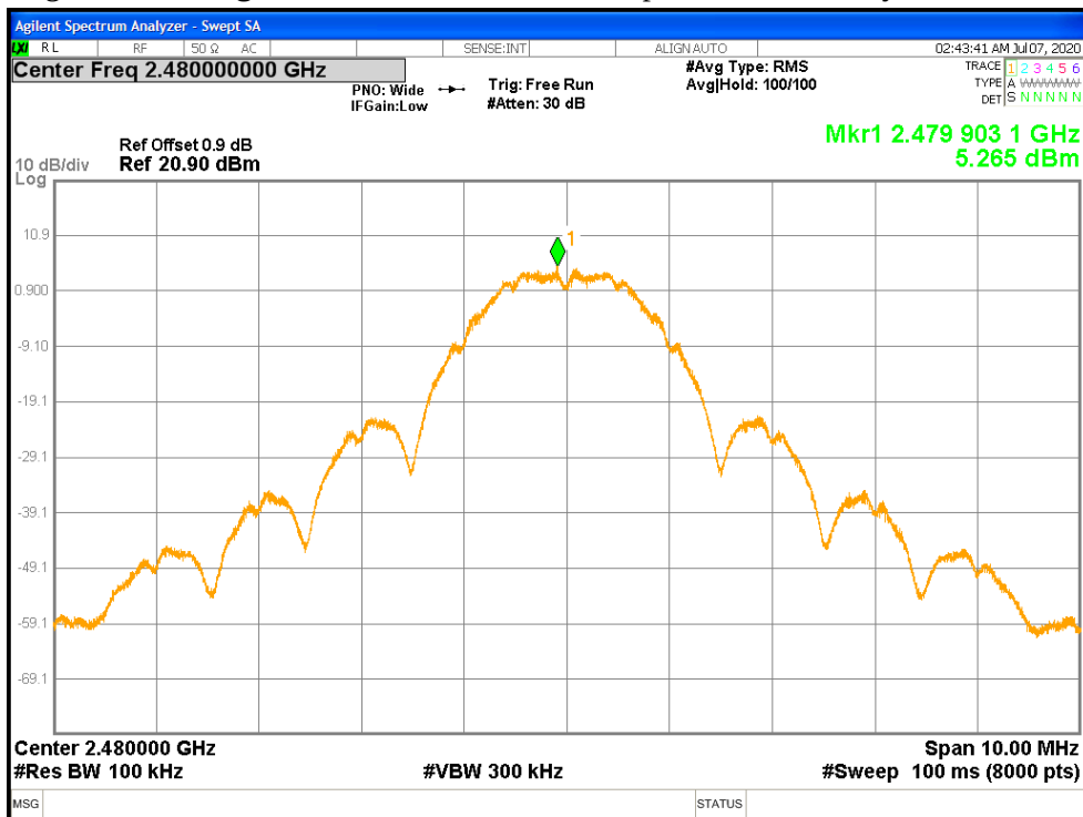
Figure 15: Zigbee Maximum Power Spectral Density-2480 MHz
