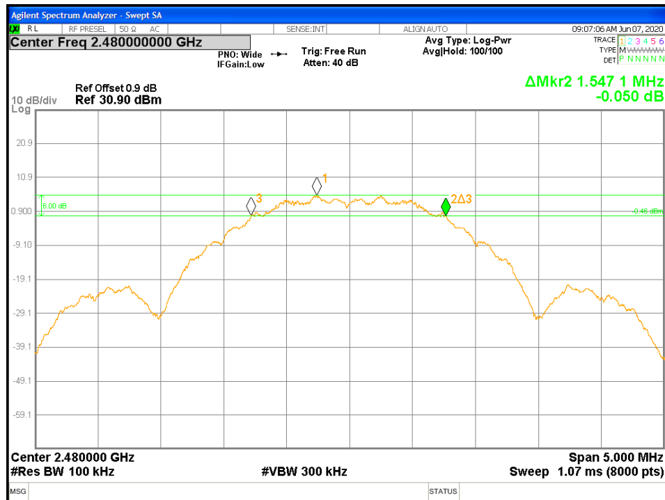
Figure 8: DTS Bandwidth-Transmitter -2480 MHz
