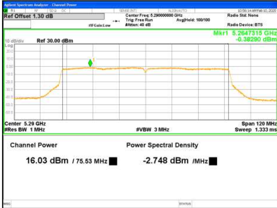
Figure 44: RMS Max Power-5290MHz-802.11ac VHT80-MCS0-TP17-2x2-CH1 (FCC)
