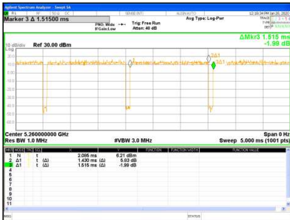
Figure 1: Duty Cycle for 802.11a at 5260MHz
