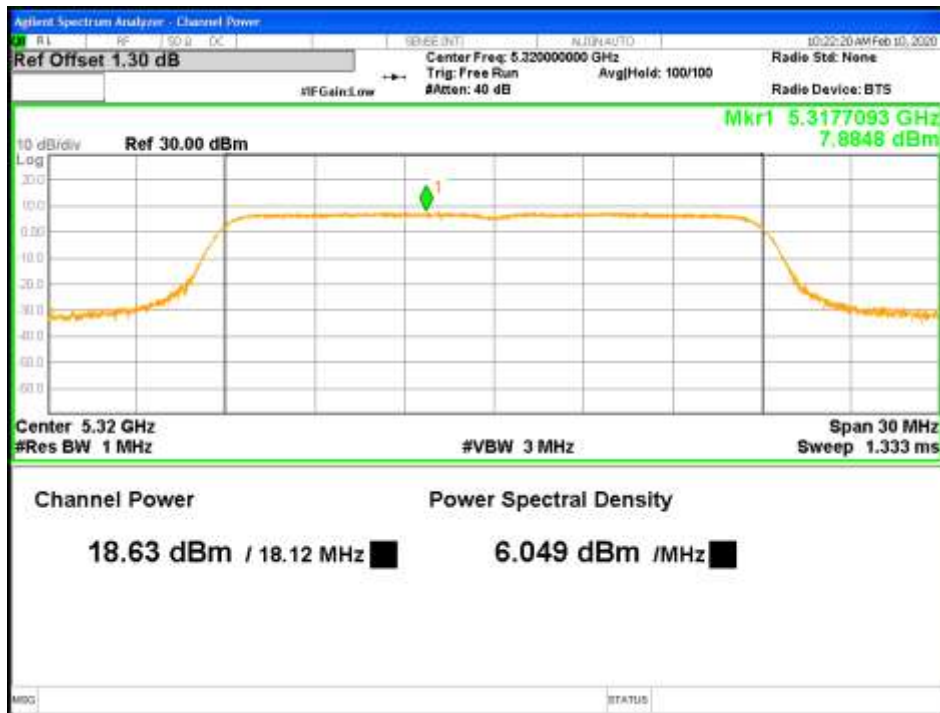
Figure 13: RMS Max Power-5320MHz-802.11ac VHT20-MCS0-TP19-1x2-CH0 (RSS)
