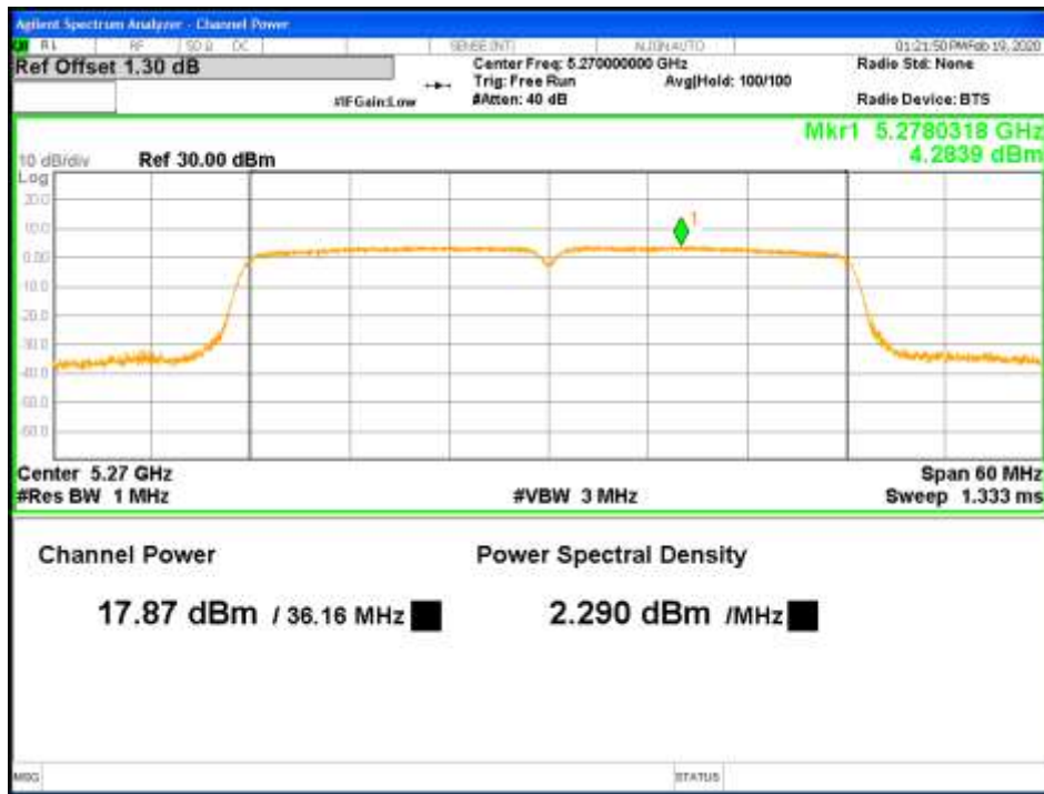
Figure 19: RMS Max Power-5270MHz-802.11ac VHT40-MCS0-TP18-1x2-CH0 (RSS)
