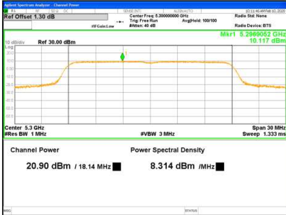
Figure 12: RMS Max Power-5300MHz-802.11ac VHT20-MCS0-TP21-1x2-CH1 (FCC)
