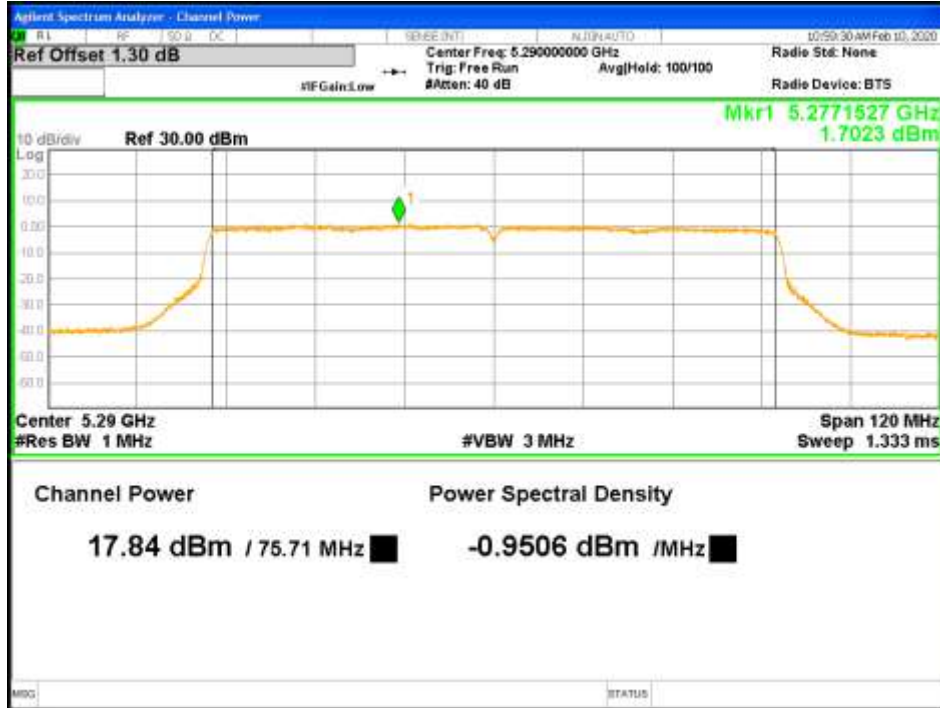
Figure 24: RMS Max Power-5290MHz-802.11ac VHT80-MCS0-TP18.5-1x2-CH1 (FCC & RSS)
