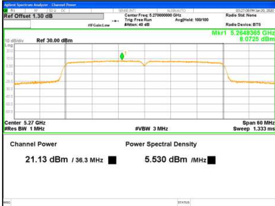
Figure 18: RMS Max Power-5270MHz-802.11ac VHT40-MCS0-TP21-1x2-CH1 (FCC)
