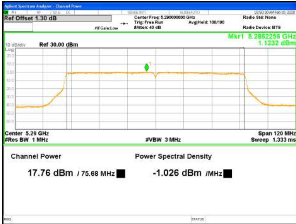
Figure 23: RMS Max Power-5290MHz-802.11ac VHT80-MCS0-TP18.5-1x2-CH0 (FCC & RSS)
