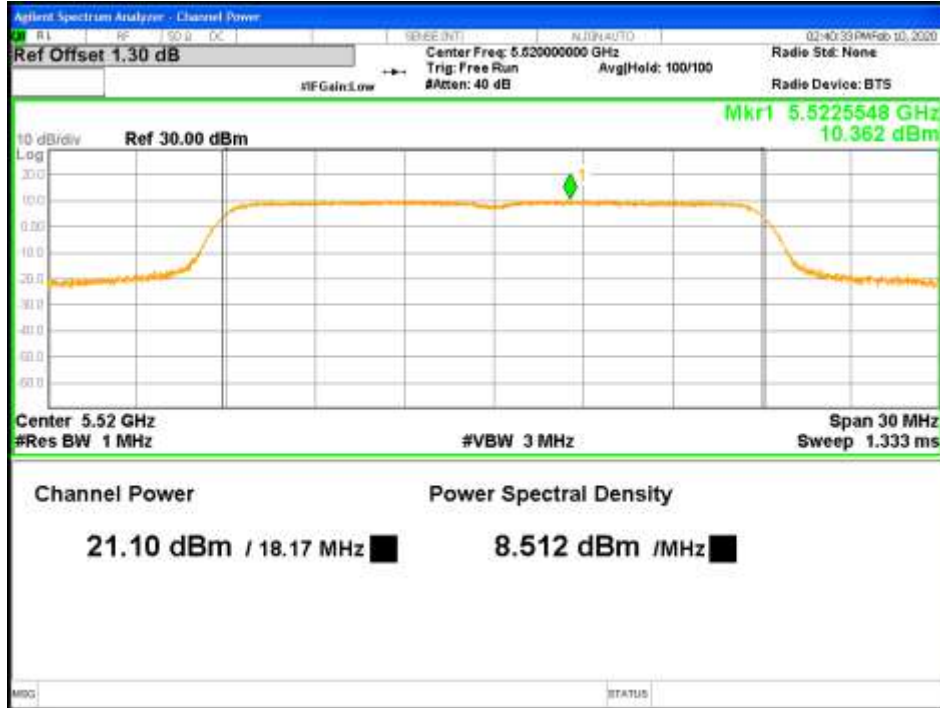
Figure 16: RMS Max Power-5520MHz-802.11ac VHT20-MCS0-TP21-1x2-CH1
