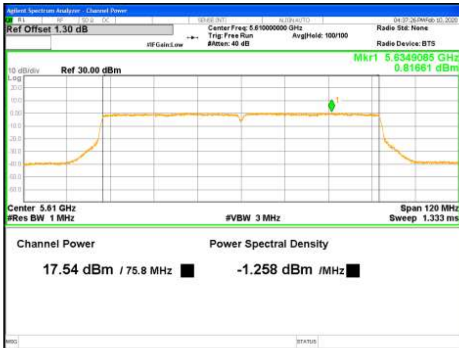
Figure 47: RMS Max Power-5610MHz-802.11ac VHT80-MCS0-TP19-2x2-CH0
