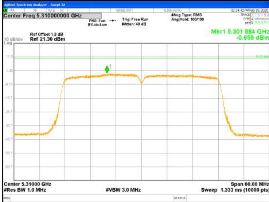
Figure 75: PPSD-5310MHz-802.11ac VHT40-MCS0-TP13-CH1-2x2 (RSS)
