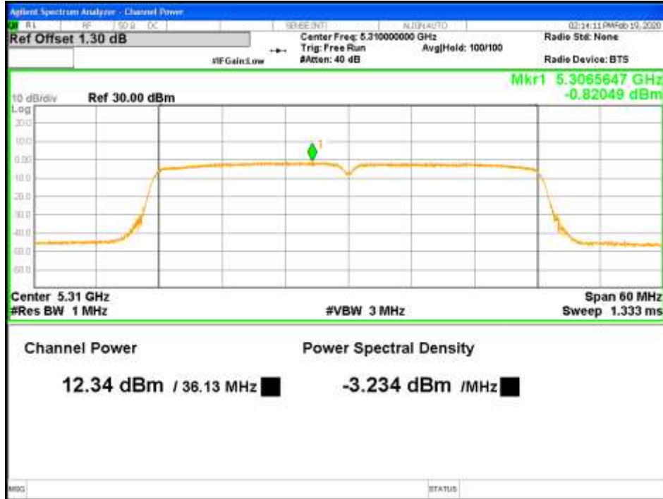
Figure 40: RMS Max Power-5310MHz-802.11ac VHT40-MCS0-TP13-2x2-CH1 (RSS)
