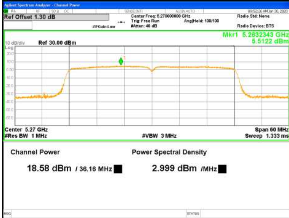
Figure 38: RMS Max Power-5270MHz-802.11ac VHT40-MCS0-TP18.5-2x2-CH1 (FCC)
