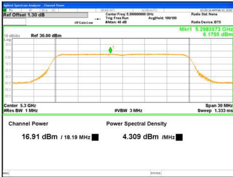
Figure 31: RMS Max Power-5300MHz-802.11ac VHT20-MCS0-TP17-2x2-CH0 (FCC)
