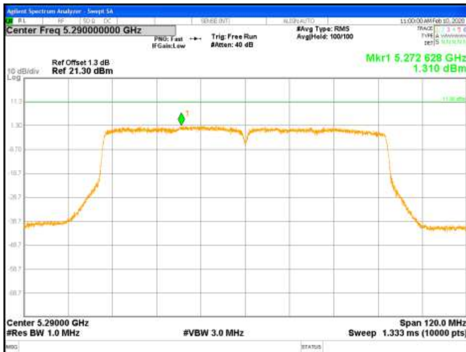
Figure 69: PPSD-5290MHz-802.11ac VHT80-MCS0-TP18.5-CH1-1x2 (FCC & RSS)
