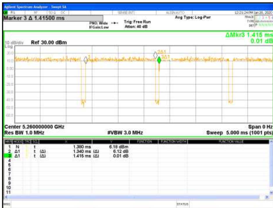
Figure 2: Duty Cycle for 802.11n HT20 and 802.11ac VHT20 at 5260MHz
