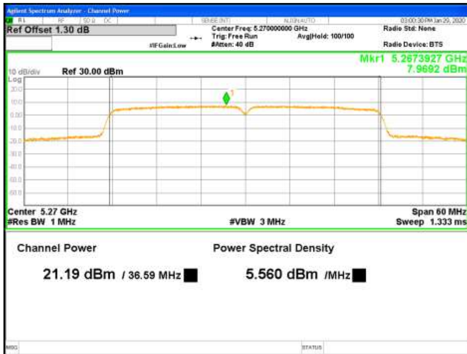
Figure 17: RMS Max Power-5270MHz-802.11ac VHT40-MCS0-TP21-1x2-CH0 (FCC)
