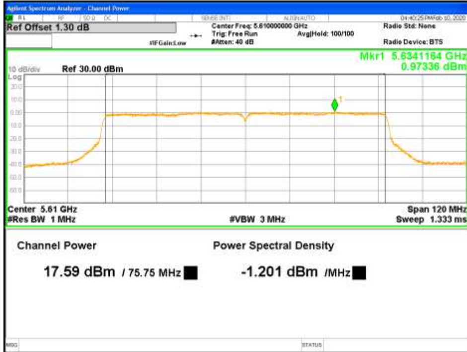
Figure 48: RMS Max Power-5610MHz-802.11ac VHT80-MCS0-TP19-2x2-CH1
