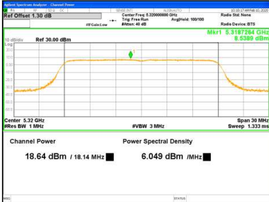
Figure 14: RMS Max Power-5320MHz-802.11ac VHT20-MCS0-TP19-1x2-CH1 (RSS)
