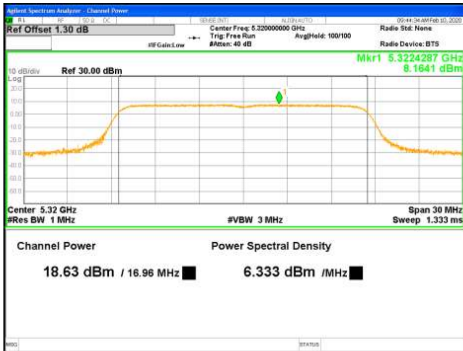
Figure 7: RMS Max Power-5320MHz-802.11a-6Mbps-TP19-1x2-CH0 (RSS)
