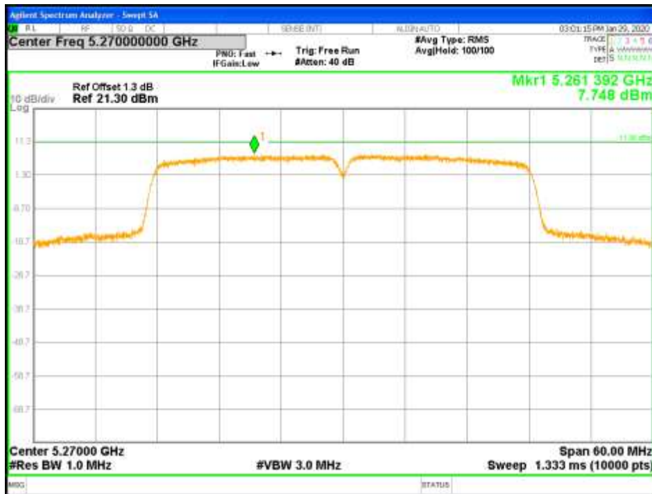
Figure 66: PPSD-5270MHz-802.11ac VHT40-MCS0-TP21-CH0-1x2 (FCC)
