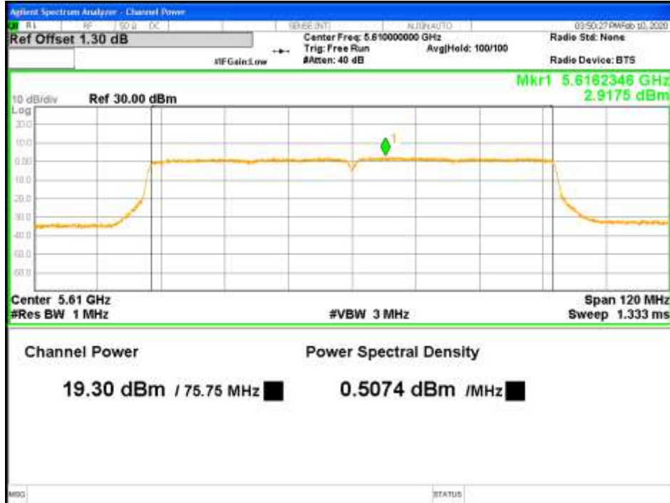
Figure 26: RMS Max Power-5610MHz-802.11ac VHT80-MCS0-TP20.5-1x2-CH1
