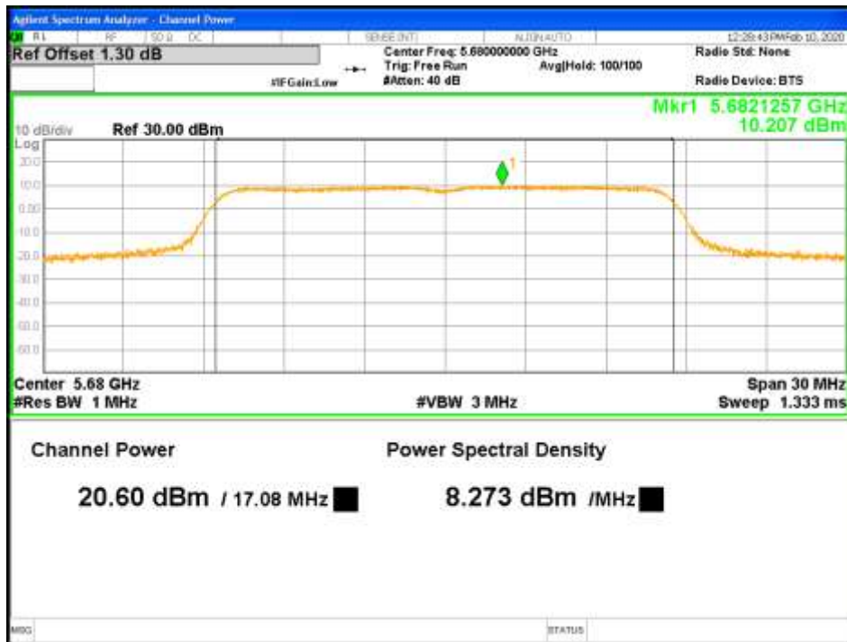
Figure 9: RMS Max Power-5680MHz-802.11a-6Mbps-TP21-1x2-CH0
