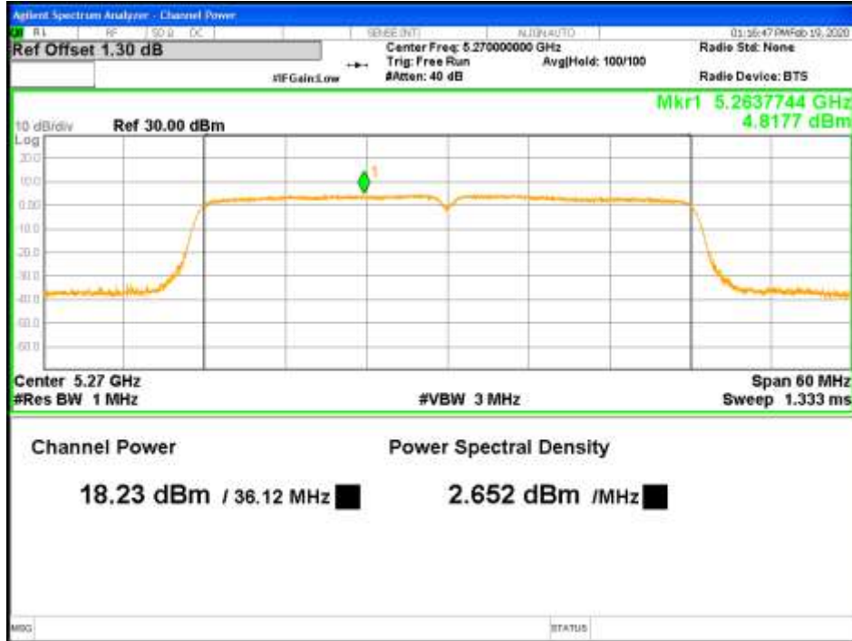
Figure 20: RMS Max Power-5270MHz-802.11ac VHT40-MCS0-TP18-1x2-CH1 (RSS)
