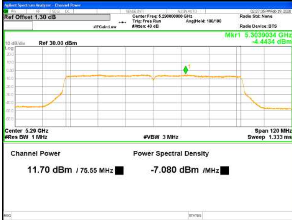
Figure 46: RMS Max Power-5290MHz-802.11ac VHT80-MCS0-TP13-2x2-CH1 (RSS)
