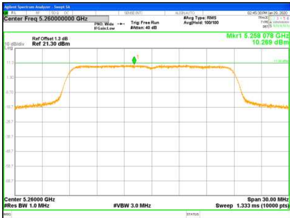
Figure 63: PPSD-5260MHz-802.11ac VHT20-MCS0-TP21-CH0-1x2 (FCC)
