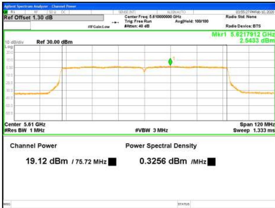
Figure 25: RMS Max Power-5610MHz-802.11ac VHT80-MCS0-TP20.5-1x2-CH0
