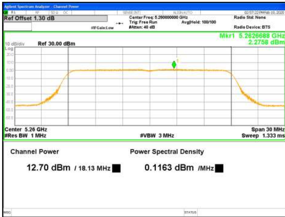
Figure 33: RMS Max Power-5260MHz-802.11ac VHT20-MCS0-TP13-2x2-CH0 (RSS)
