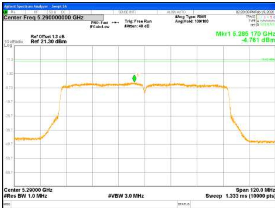
Figure 78: PPSD-5290MHz-802.11ac VHT80-MCS0-TP13-CH1-2x2 (RSS)
