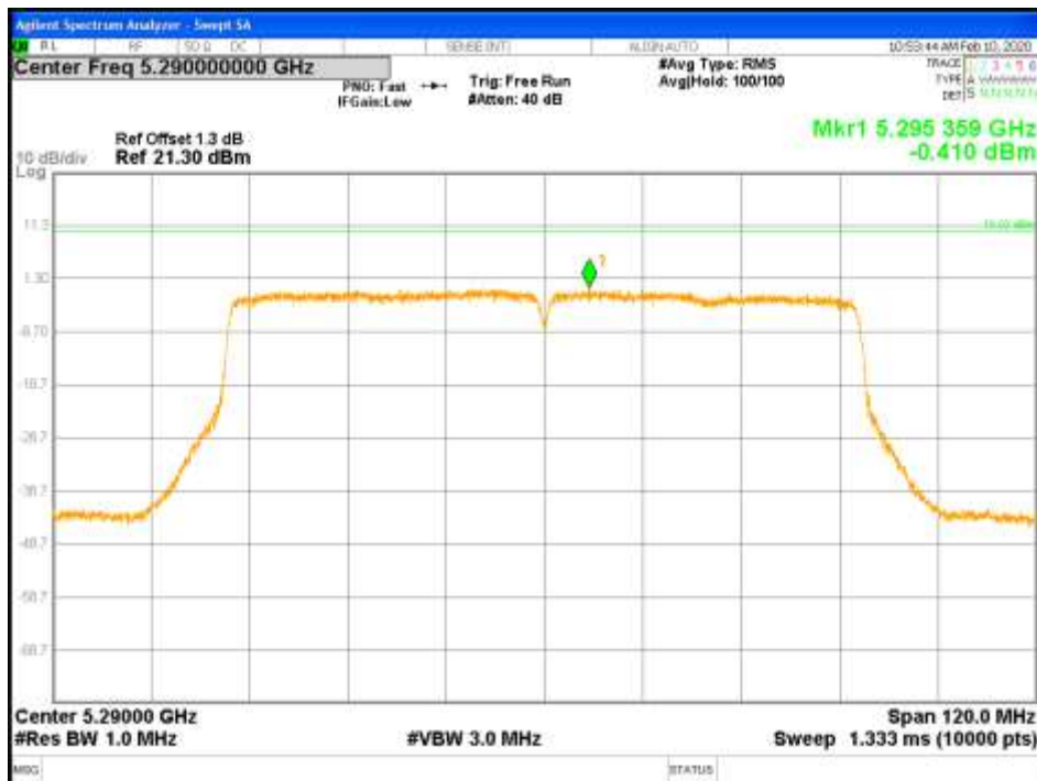
Figure 77: PPSD-5290MHz-802.11ac VHT80-MCS0-TP17-CH0-2x2 (FCC)
