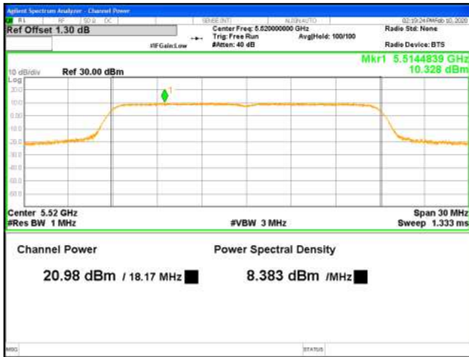
Figure 15: RMS Max Power-5520MHz-802.11ac VHT20-MCS0-TP21-1x2-CH0
