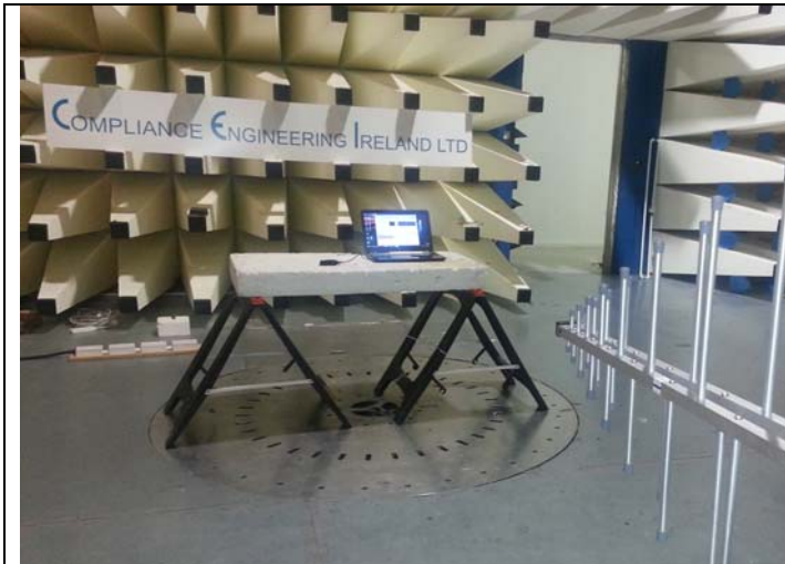
Fig 1 Radiated Emissions 30M -1GHz-
