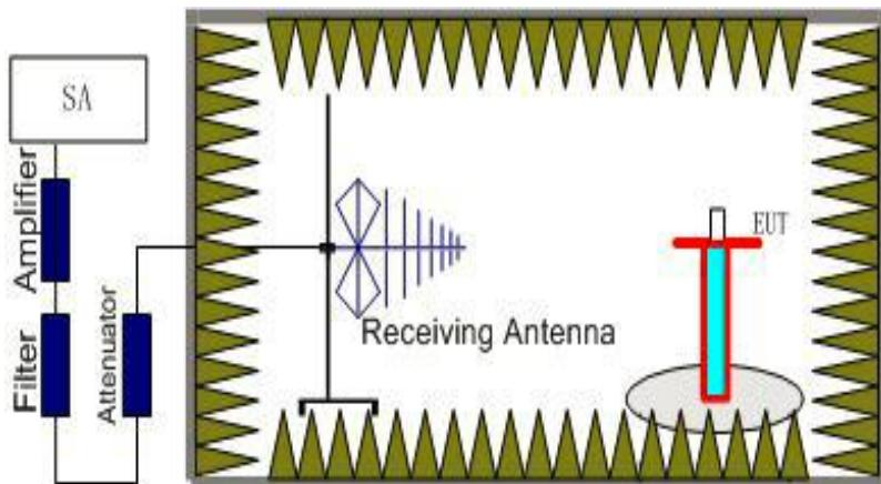
2. The EUT is then put into continuously transmitting mode at its maximum power level during the test. And the maximum value of the receiver should be recorded as  $(P_r)$ .
