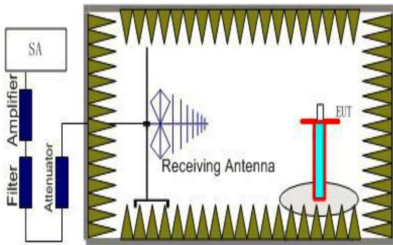
2. The EUT is then put into continuously transmitting mode at its maximum power level during the test. And the maximum value of the receiver should be recorded as (Pr).
