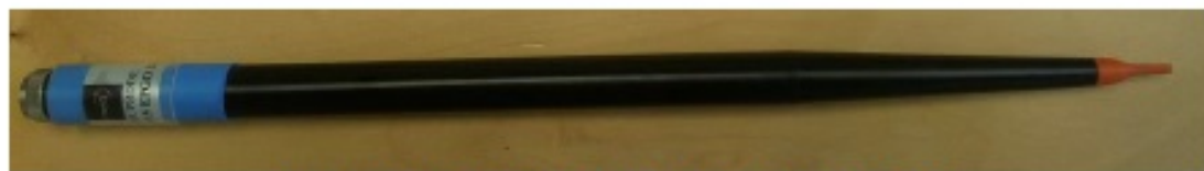
Figure 1 – MVG COMOSAR Dosimetric E field Dipole
