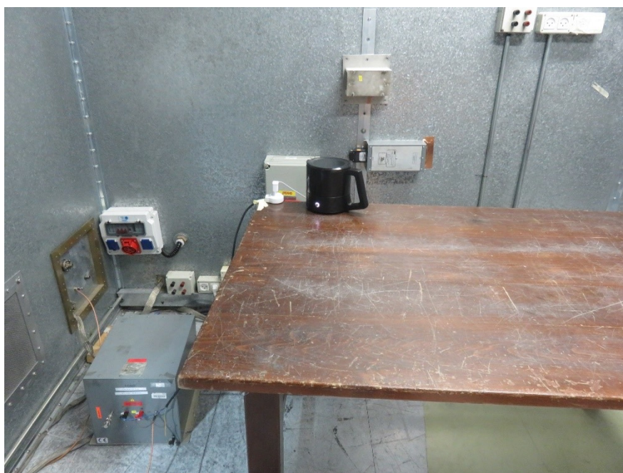
Photograph 4: Conducted Emission Testing on AC Power Supply Port
