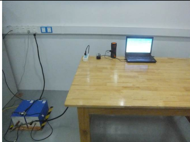
Conducted Emissions Test Setup – Front View
