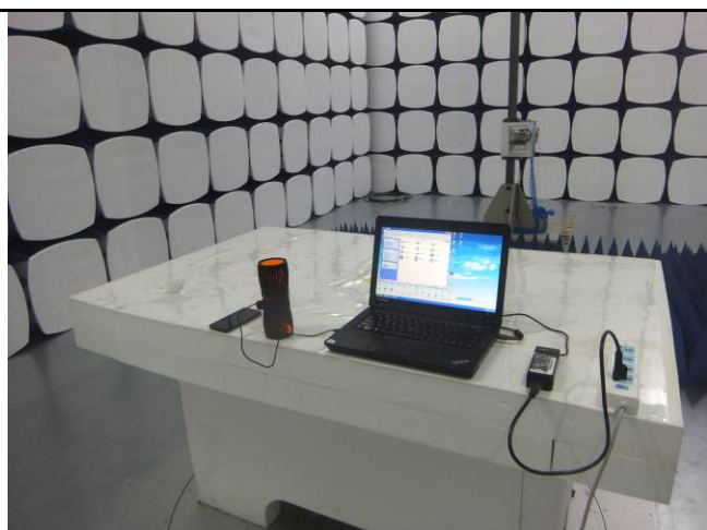
Radiated Spurious Emissions Test Setup Above 1GHz
