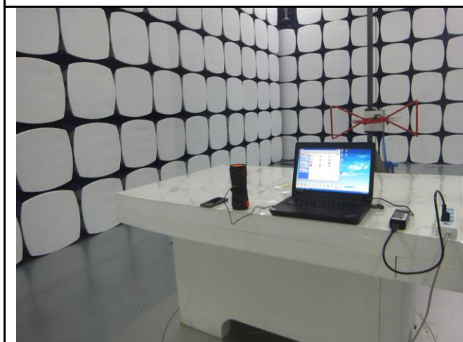
Conducted Emissions Test Setup – Front View
