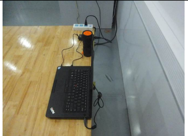
Conducted Emissions Test Setup Side View
