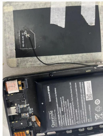
Antenna mounting position
