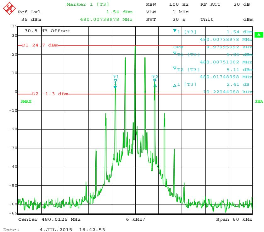
**Emission Mask D with High Power 12.5 kHz, 480.0125 MHz**
