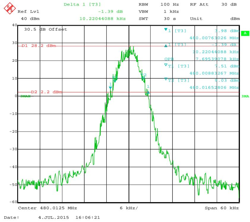
**99% Occupied Bandwidth & 26 dB Emissions Bandwidth 12.5 kHz, 480.0125 MHz (Low Power)**
