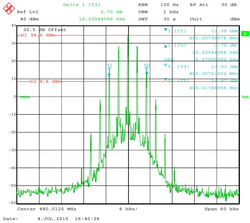
**99% Occupied Bandwidth & 26 dB Emissions Bandwidth 12.5 kHz, 480.0125 MHz (Low Power)**
