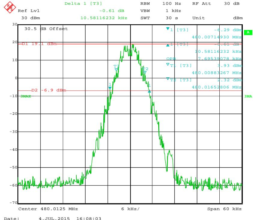
**Emission Mask D with High Power 12.5 kHz, 480.0125 MHz**
