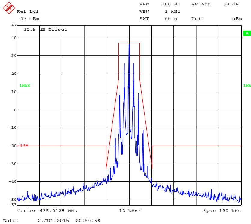
**Emission Mask D with Low Power 12.5 kHz, 435.0125 MHz**
