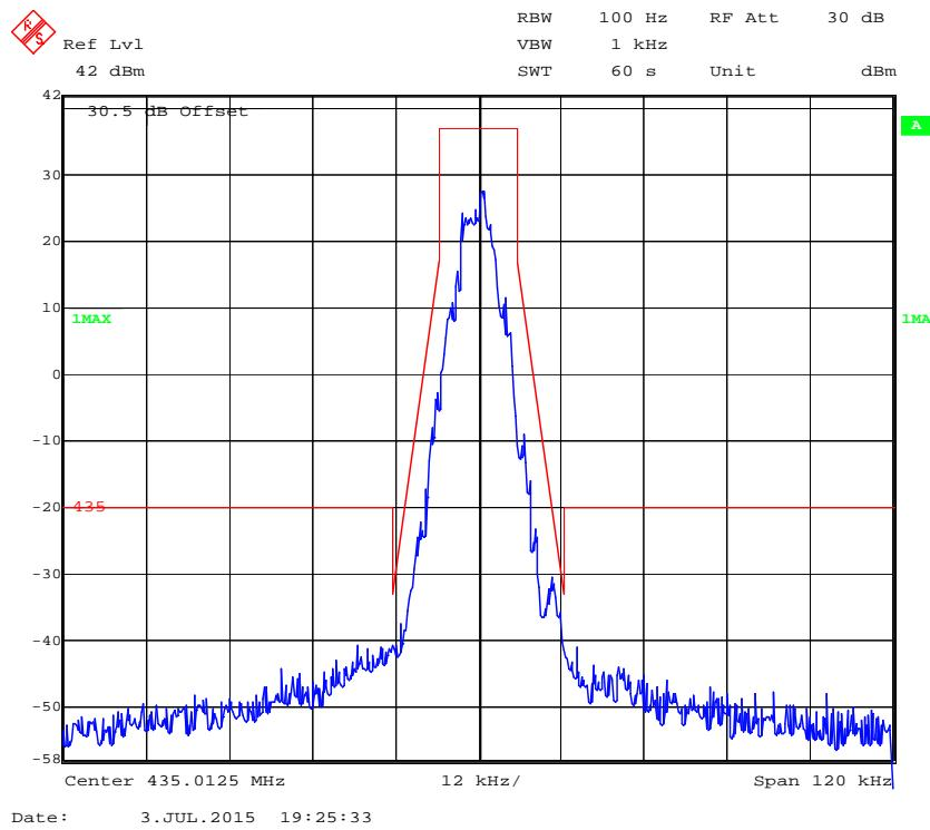
**Emission Mask D with Low Power 12.5 kHz, 435.0125 MHz**
