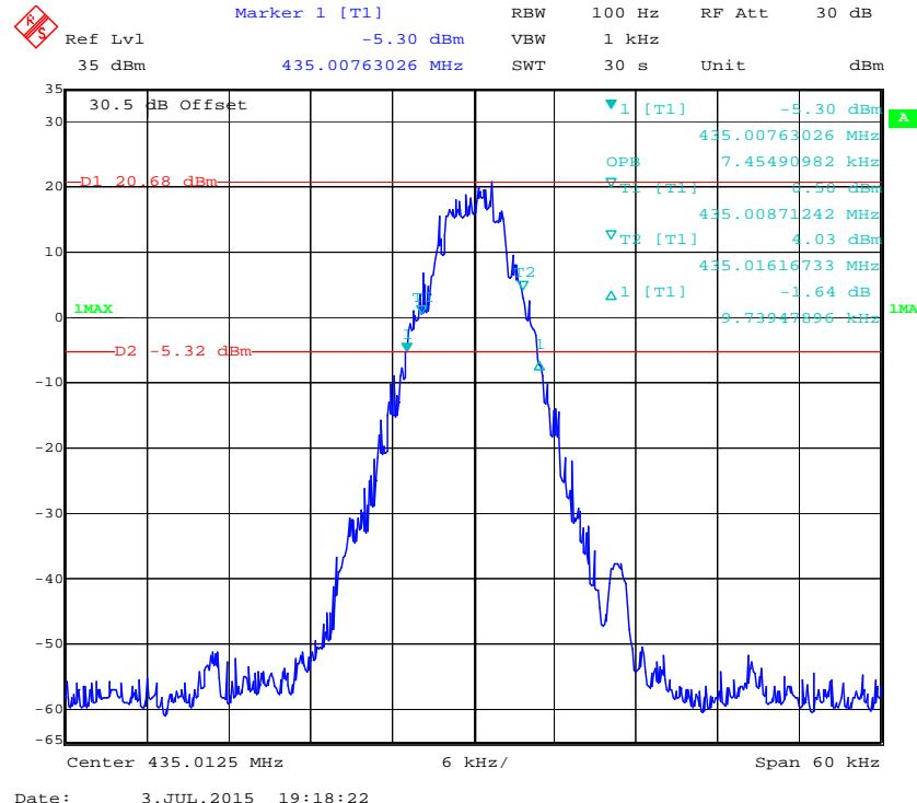
**Emission Mask D with High Power 12.5 kHz, 435.0125 MHz**
