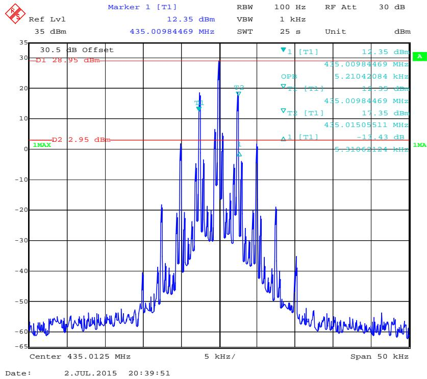
**Emission Mask D with High Power 12.5 kHz, 435.0125 MHz**
