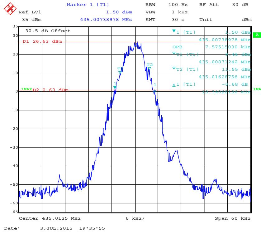
**99% Occupied Bandwidth & 26 dB Emissions Bandwidth 12.5 kHz, 435.0125 MHz (Low Power)**
