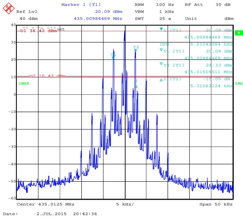
**99% Occupied Bandwidth & 26 dB Emissions Bandwidth 12.5 kHz, 435.0125 MHz (Low Power)**
