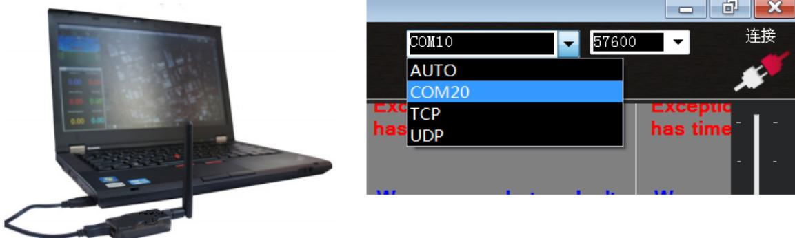
Use the micro-USB cable to connect the ground module to your laptop. In Mission Planner and APM Planner ground station applications, select the communication option that shows COM, set the rate to 57600, and select Connect. The radio will not connect unless the vehicle is powered. Use the Flight Data screen to view your vehicle's status and control missions in flight.
