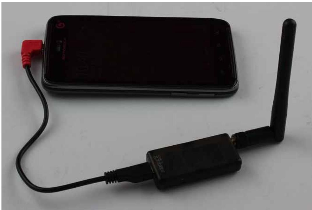
Connect the HTOX-G ground module to your tablet using the Android adapter cable. Connect the red end to the tablet and the black end to the radio. In DroidPlanner or Andropilot, select Connect.
