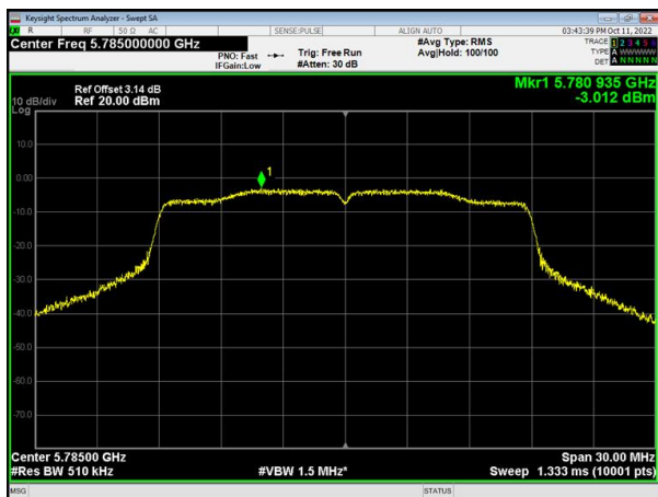
(802.11ac20) PSD plot on channel 165
