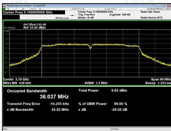
(802.11 ac40) 99% Bandwidth plot on channel 42
