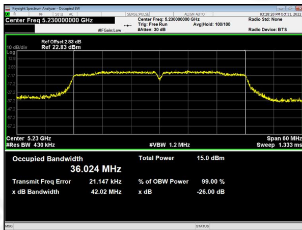
(802.11 ac40) 99% Bandwidth plot on channel 42
