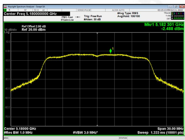
(802.11n20) PSD plot on channel 40
