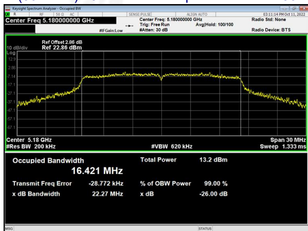
(802.11 a) 26dB Bandwidth plot on channel 36
