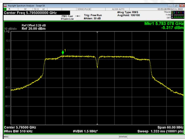
(802.11ac40) PSD plot on channel 159
