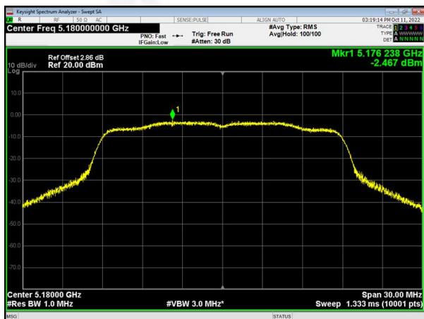
(802.11ac20) PSD plot on channel 40
