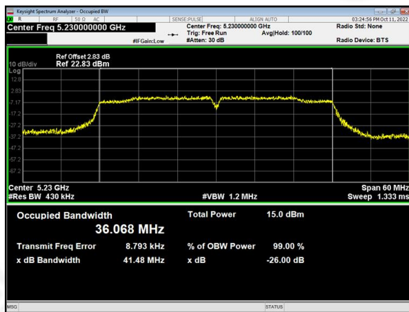
(802.11 n40) 26dB Bandwidth plot on channel 46
