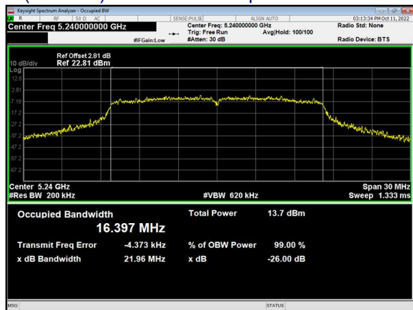
(802.11 a) 26dB Bandwidth plot on channel 48
