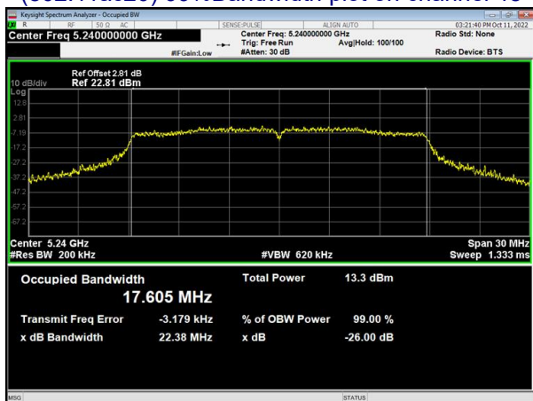
(802.11ac20) 99%Bandwidth plot on channel 48
