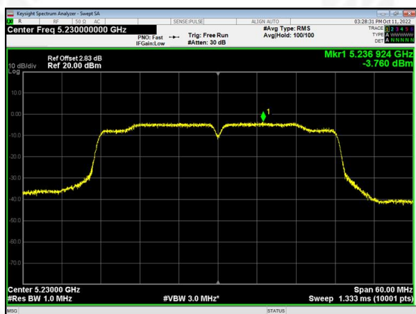
(802.11ac40) PSD plot on channel 46
