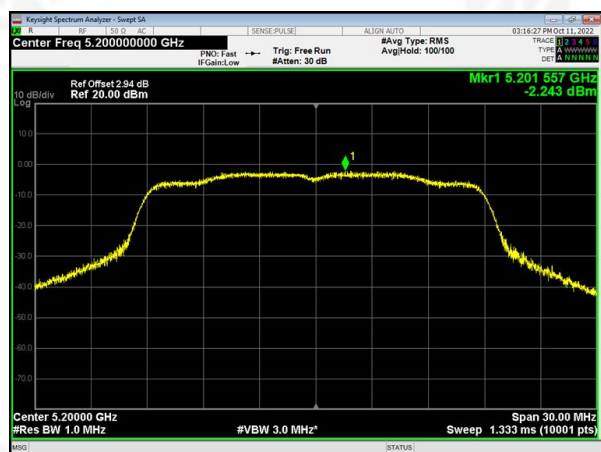
(802.11n20) PSD plot on channel 40
