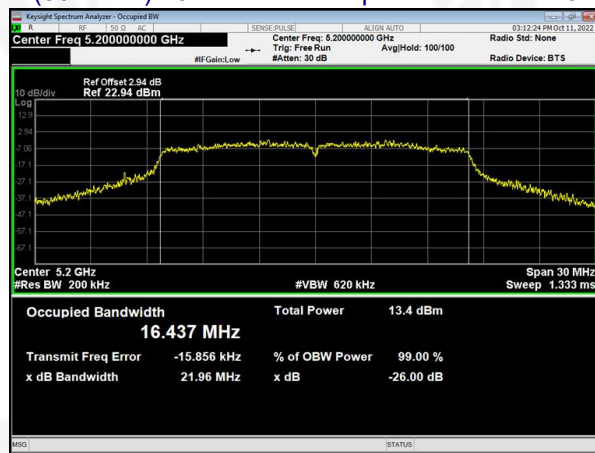
(802.11 a) 26dB Bandwidth plot on channel 40
