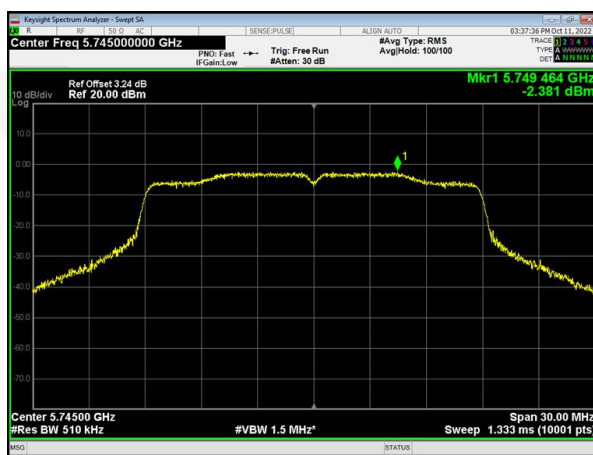
(802.11n20) PSD plot on channel 157
