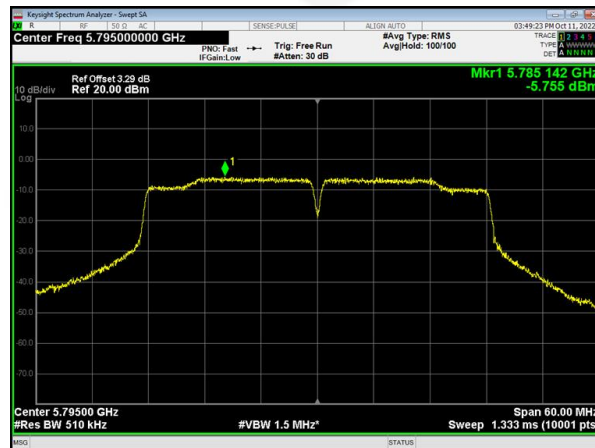
(802.11n40) PSD plot on channel 159
