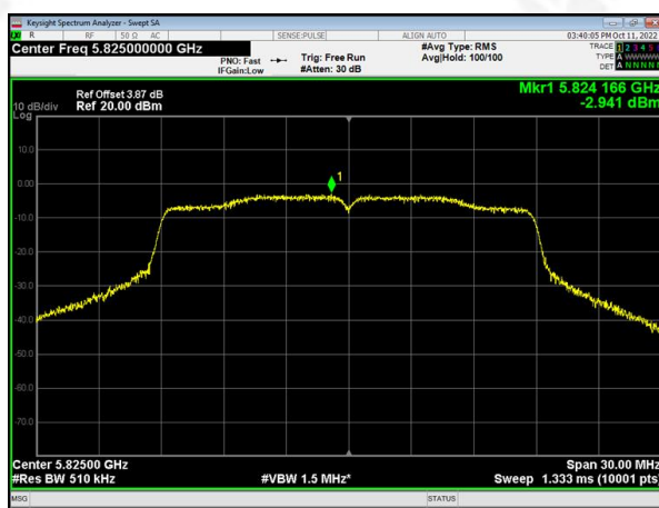
(802.11n20) PSD plot on channel 165
