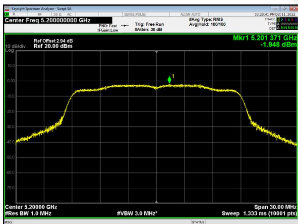
(802.11ac20) PSD plot on channel 40
