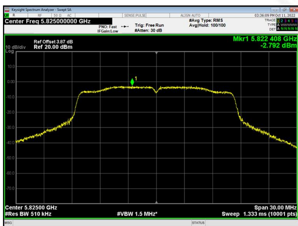
(802.11a) PSD plot on channel 165
