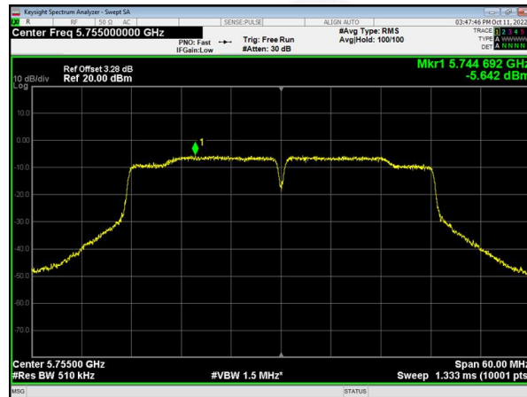
ANT (802.11n40) PSD plot on channel 151
