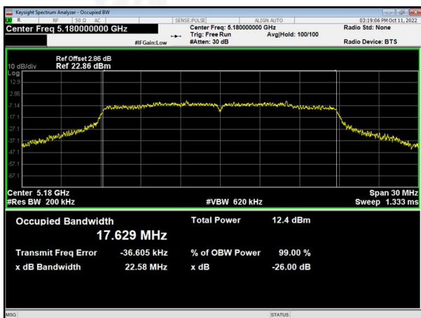
(802.11ac20) 99%Bandwidth plot on channel 40
