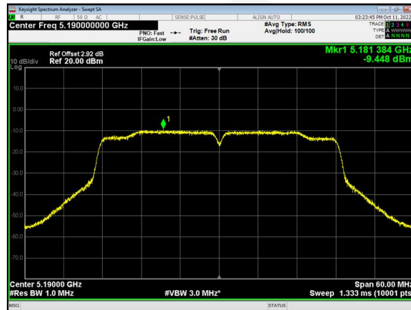
(802.11n40) PSD plot on channel 46
