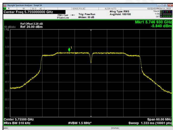
(802.11ac40) PSD plot on channel 159
