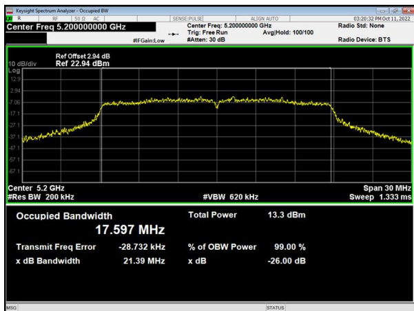
(802.11ac20) 99%Bandwidth plot on channel 48
