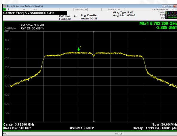
(802.11n20) PSD plot on channel 157
