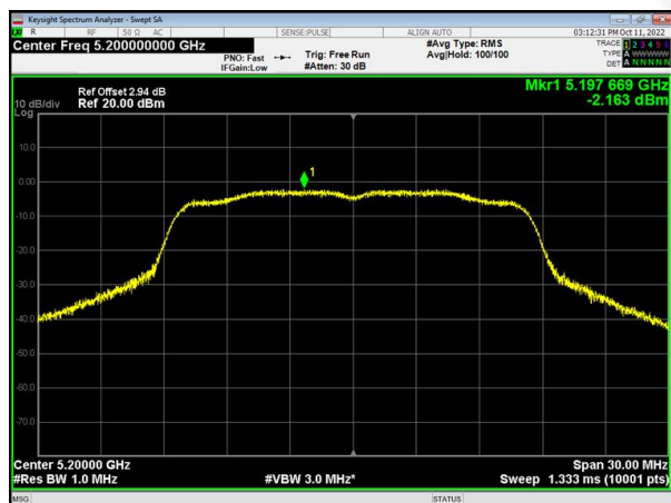
(802.11a) PSD plot on channel 40
