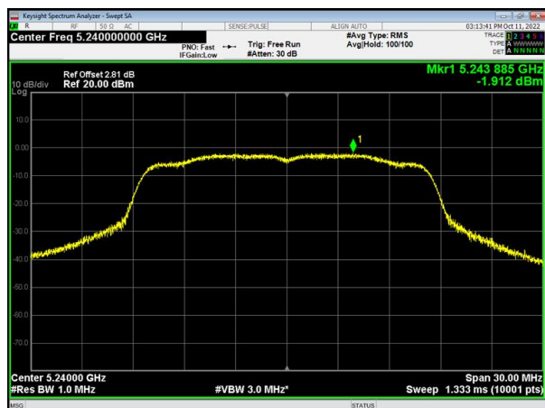
(802.11a) PSD plot on channel 48
