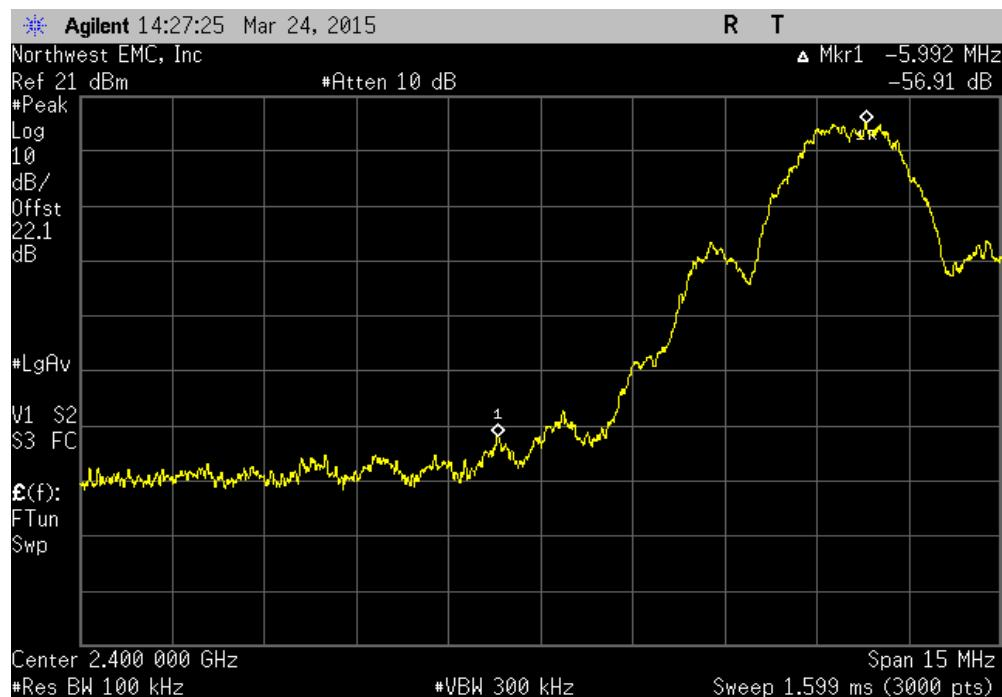
2400 MHz - 2483.5 MHz Band, High Channel 2480 MHz
