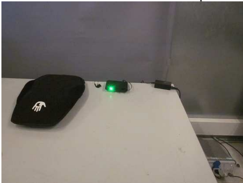
Measurement of Conducted Emission Test Set Up
