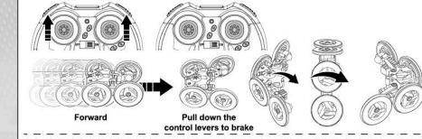
2. Backward: Pull up the left and right control levers at the same time and the car will move backward; push up the control levers at the same time and the car will flip over.
