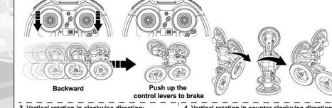
3. Vertical rotation in clockwise direction: Push up the left control lever and pull down the right lever at the same time. The car will rotate fast vertically in clockwise direction.
