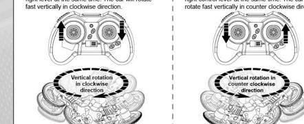
4. Vertical rotation in counter clockwise direction: Pull down the left control lever and push up the right control lever at the same time. The car will rotate fast vertically in counter clockwise direction.
