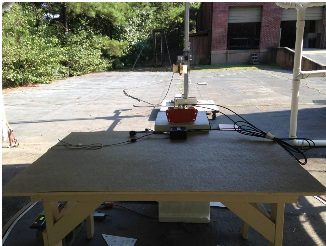
Figure 5. Radiated Emission Test Setup, above 1 GHz, Back
