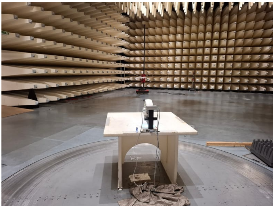
Photo 13: Semi-anechoic chamber setup
