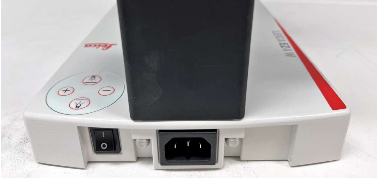
EZ4 W: - Rear view Appliance Inlet and Mains switch
