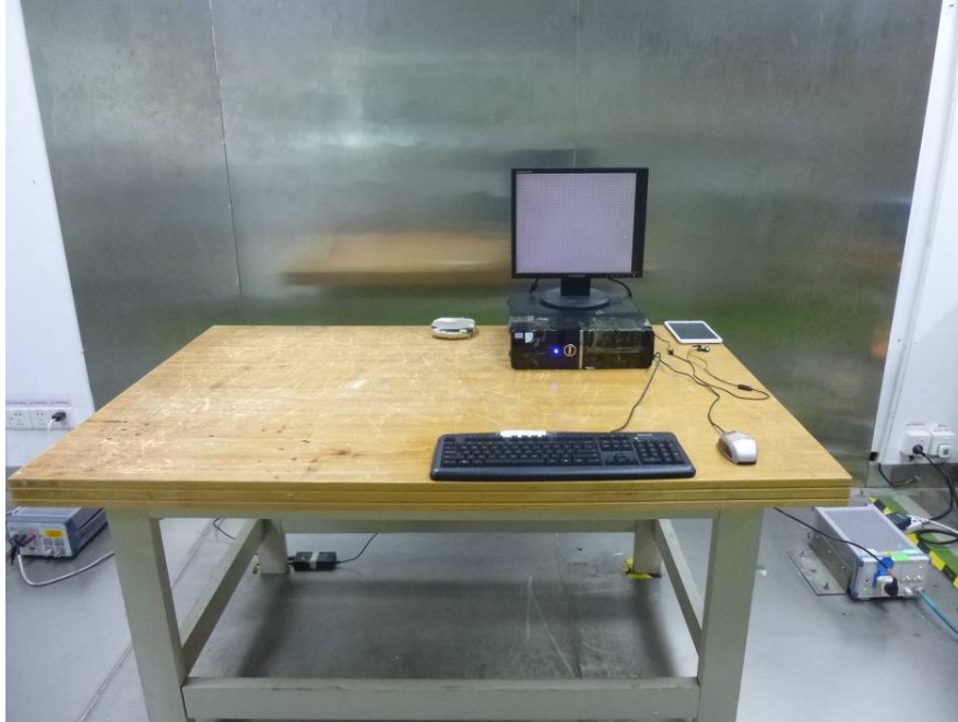
Conducted Emissions - Front View
