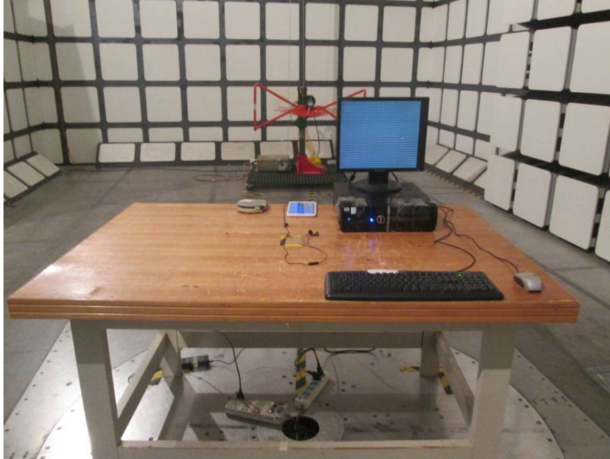
Radiated Emissions – Front View (Below 1 GHz)
