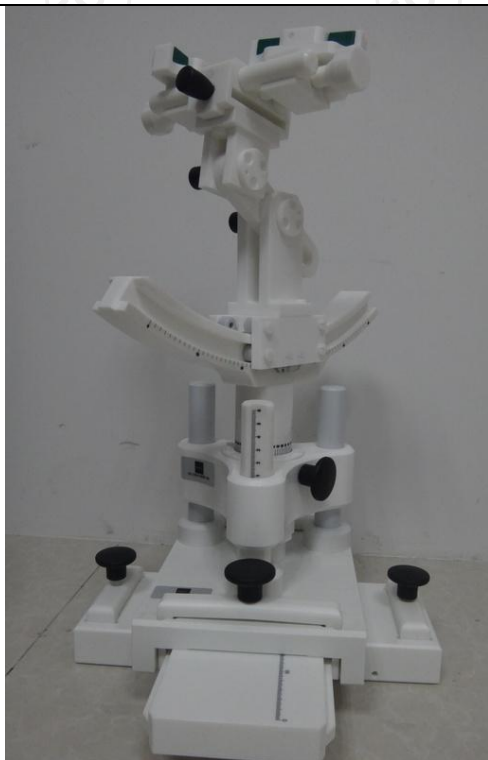
COMOSAR Mobile phone positioning system
