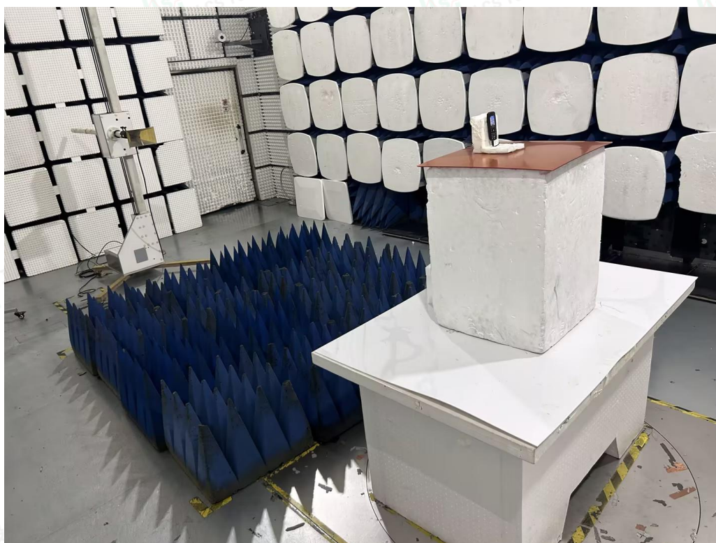
Radiated Emissions Measurement (Above 1GHz)
