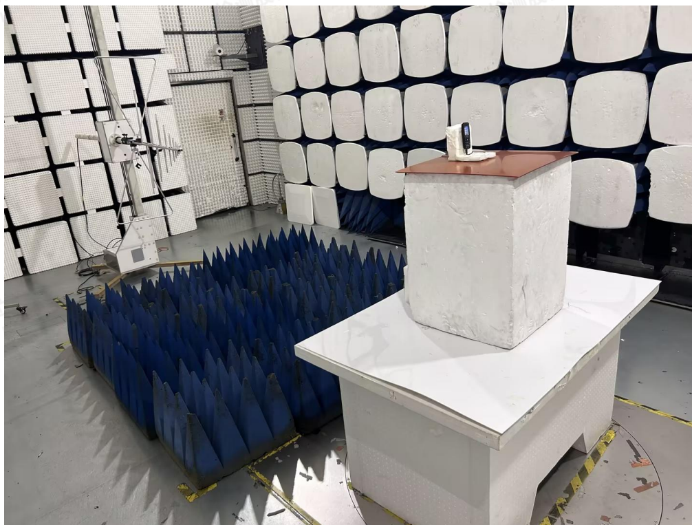
Radiated Emissions Measurement (Below 1GHz)
