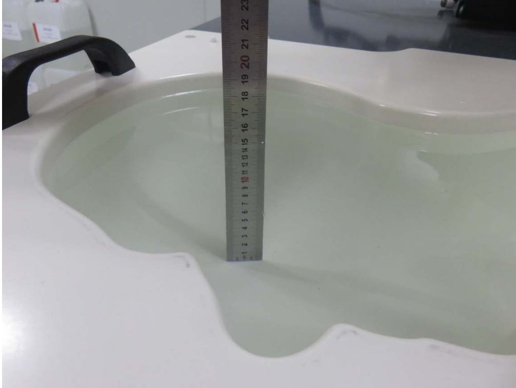
Photograph of the depth in the Head Phantom (835MHz, 15.1cm depth)
