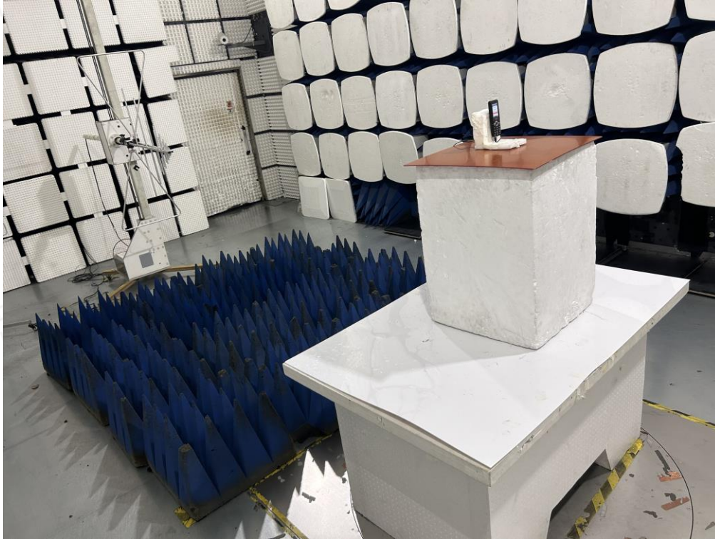
Radiated Emissions Measurement (Below 1GHz)
