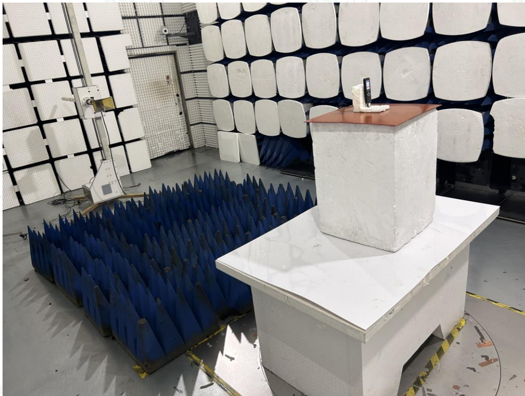
Radiated Emissions Measurement (Above 1GHz)
