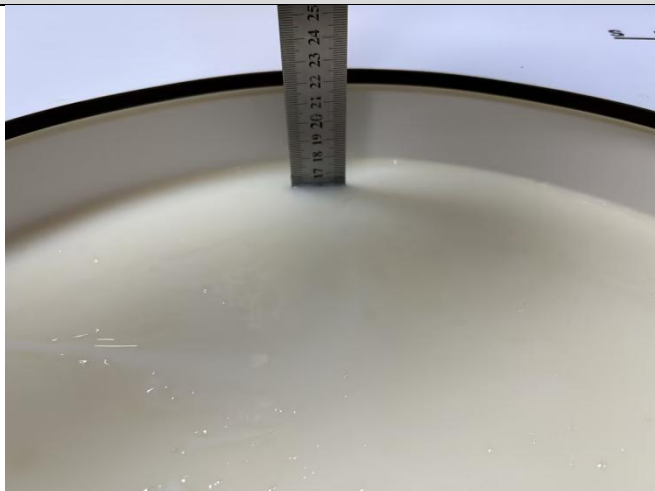
Photo 1: Tissue Simulant Liquid for Head 700-3000MHz
