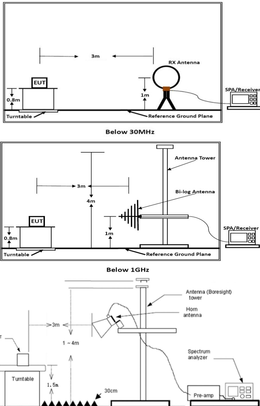
Above 10 GHz shall be extrapolated to the specified distance using an extrapolation factor of 20 dB/decade from 3m to 1.5m.
