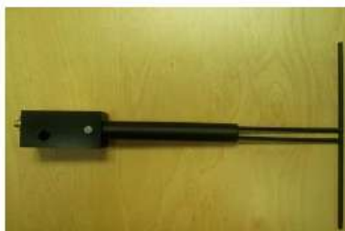
Figure 1 – MVG COMOSAR Validation Dipole
