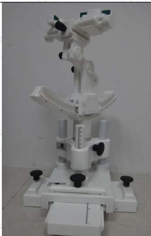
COMOSAR Mobile phone positioning system
