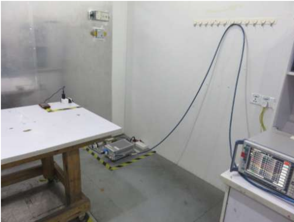
FCC RADIATED EMISSION TEST SETUP
