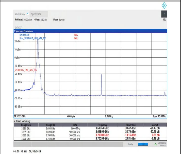
NTNV-DC_26A-n78A(3700-3800)-PC3-30-5+60-M+L-QPSK-IDLE -DFT-BPSK-Edge_1RB_Left-FAIL
