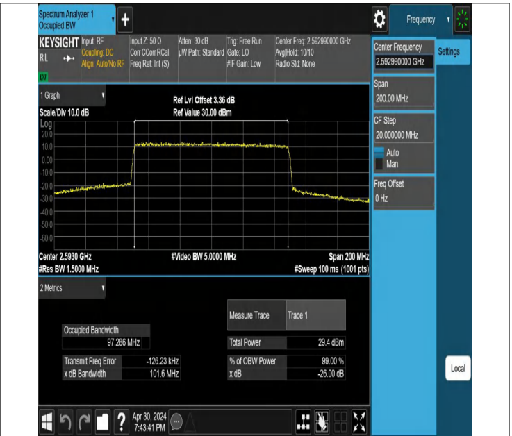
NTNV-N41-PC3-30-100-M-CP-16QAM-Outter_Full-Ant1-PASS
