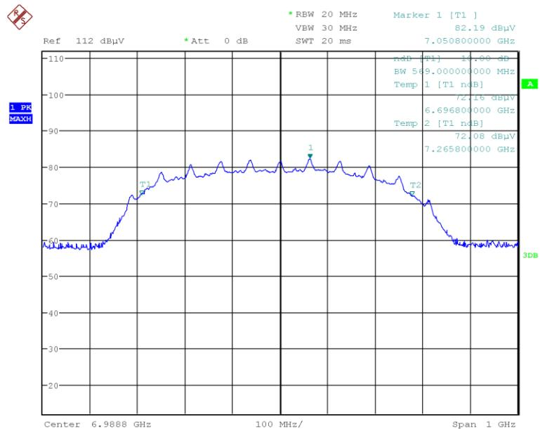
**Channel 9 (7987.2 MHz), 10dB Bandwidth****Mode 4**
