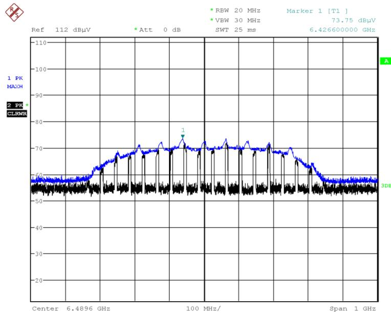
**Channel 6 (6988.8MHz), Fundamental Peak Measurements****Mode 4**
