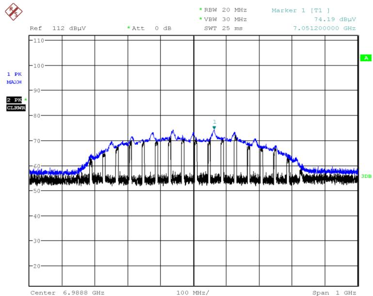
**Channel 9 (7987.2 MHz), Fundamental Peak Measurements****Mode 4**
