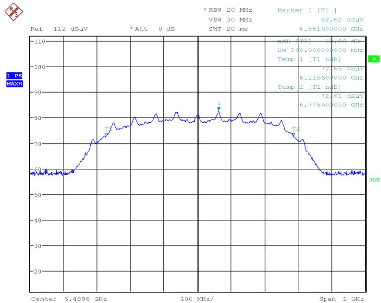
**Channel 6 (6988.8 MHz), 10dB Bandwidth****Mode 4**
