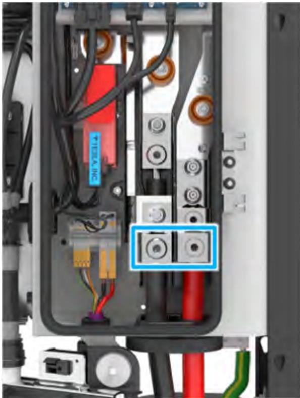
21. Use an 8 mm Hex drive with a 150 mm extension to fasten the lug set screws. Torque the lug set screws to 60Nm. Do not apply torque marks to the lugs.
