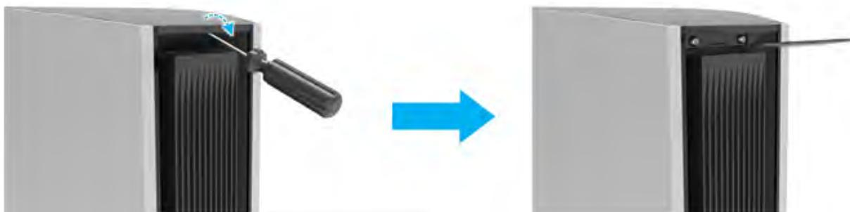
3. Use a torque driver to remove the two T27 Torx bolts securing the charge post lid to the charge post. Repeat for the other side of the charge post.
