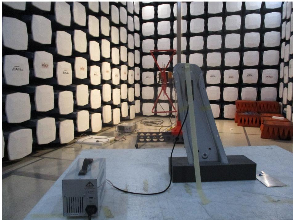
**1.6. EUT Test Setup at 3 Meters Rear View (30 MHz – 1 GHz)**
