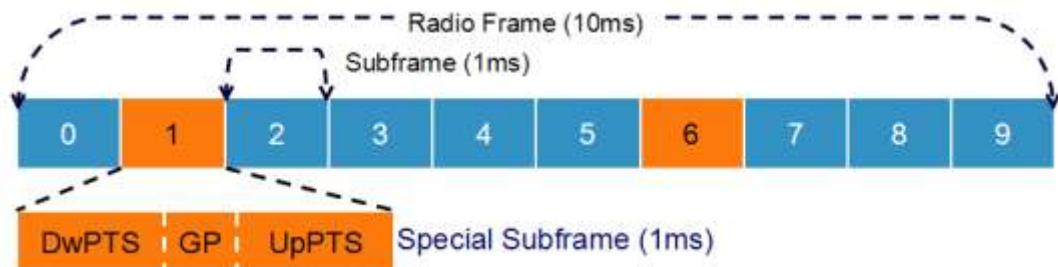
In TD-LTE frame structure, each radio frame spans 10ms and consists of ten 1ms subframes. Subframes 0 and 5 contain synchronization signal and broadcast information which is necessary for the UE to perform synchronization and obtain relevant system information.
