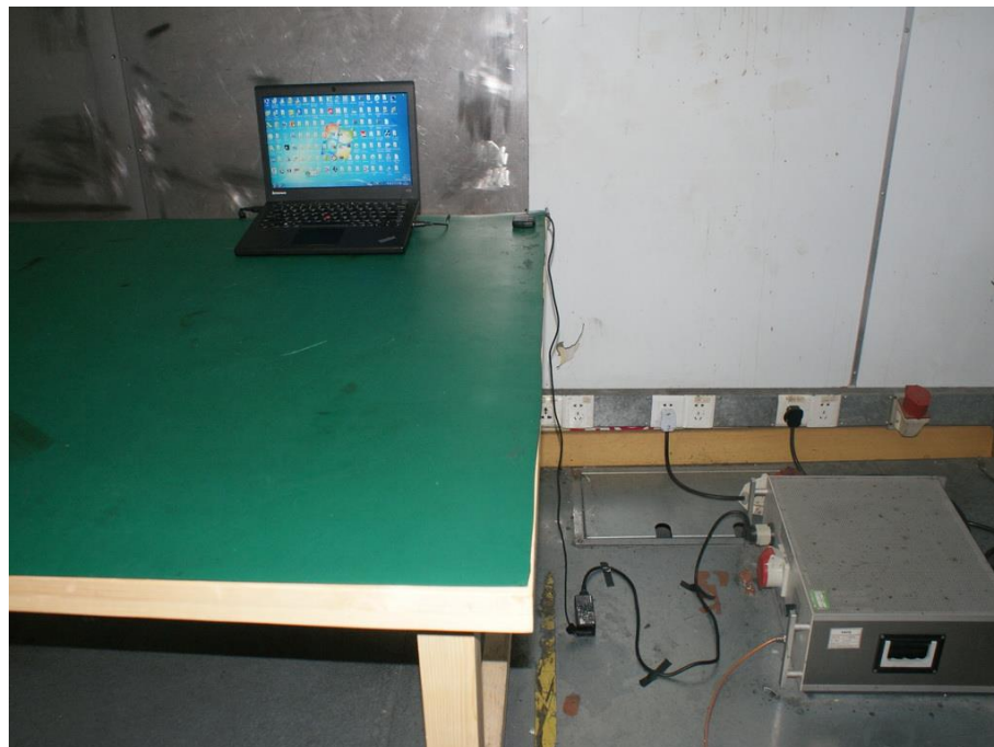
Photograph 6: Set-up for Conducted Emission on AC Mains
