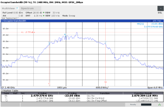
Figure 8.7-6: 99% occupied bandwidth, GFSK, 2 Mbps, 2480 MHz
