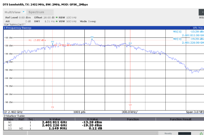
Figure 8.3-4: Minimum 6 dB bandwidth, GFSK, 2 Mbps, 2402 MHz
