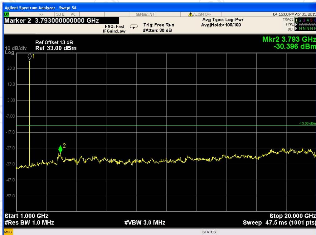
Conducted Spurious Emission on Channel 661
