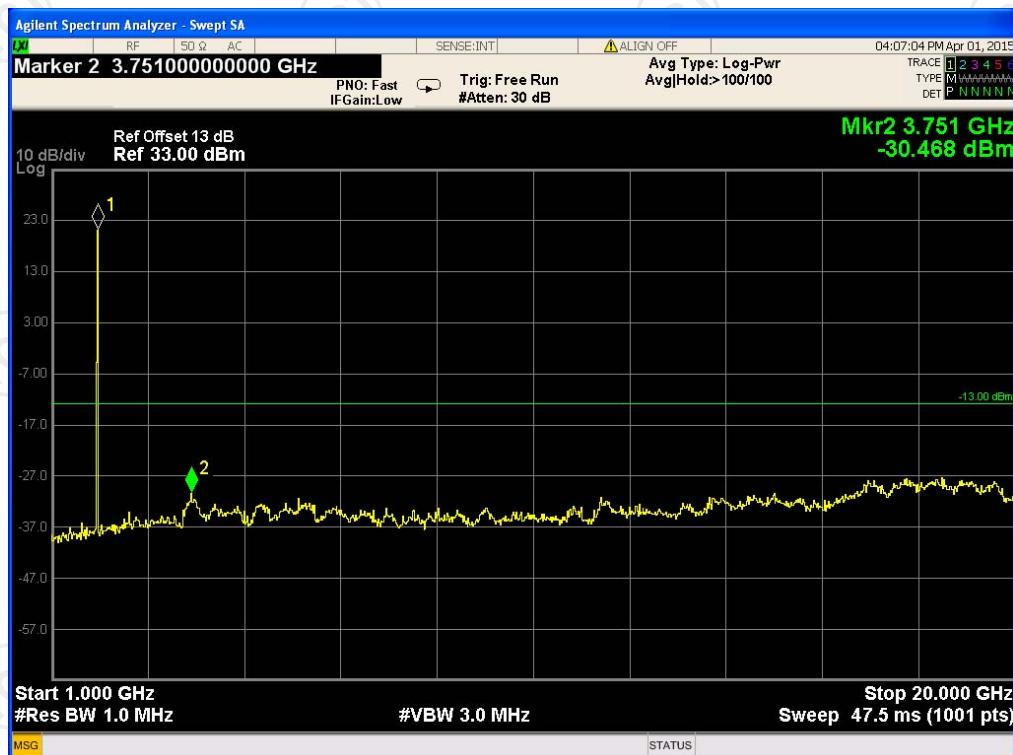
Conducted Spurious Emission on Channel 661
