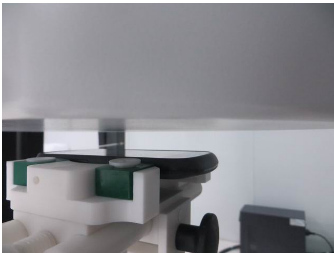
15mm body-worn Back Side Setup Photo
