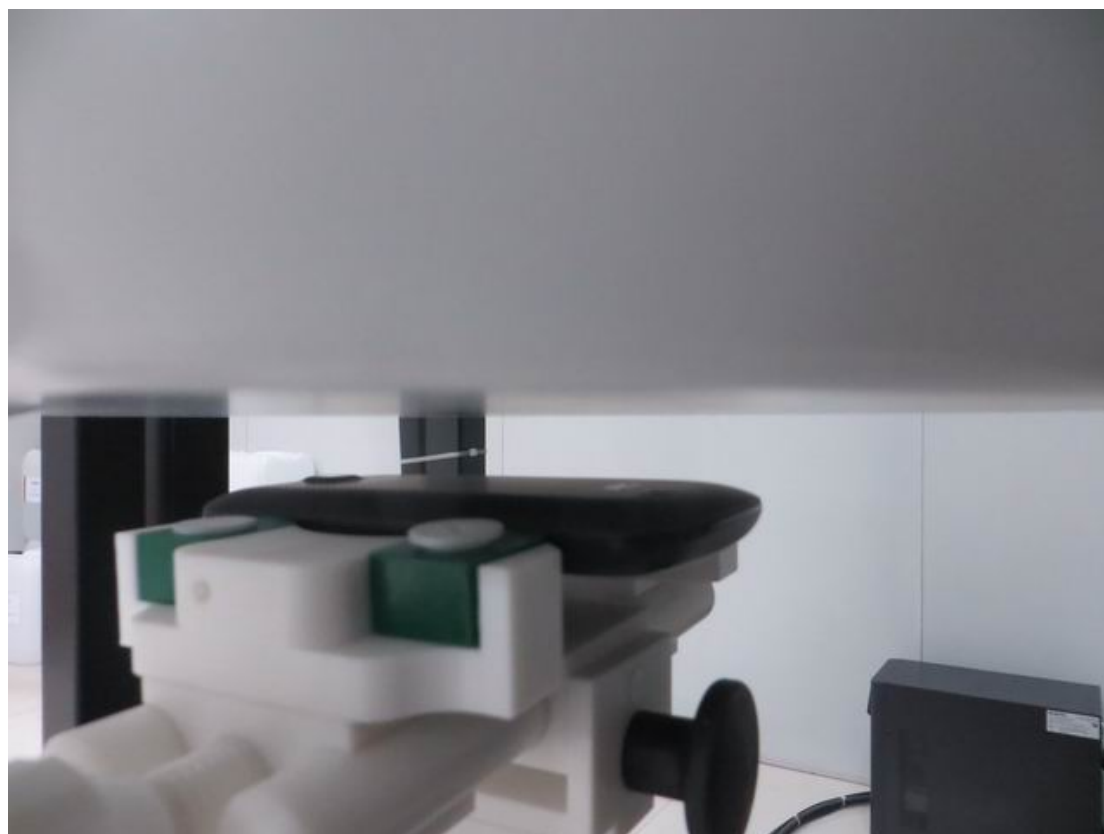
15mm body-worn Back Side Setup Photo
