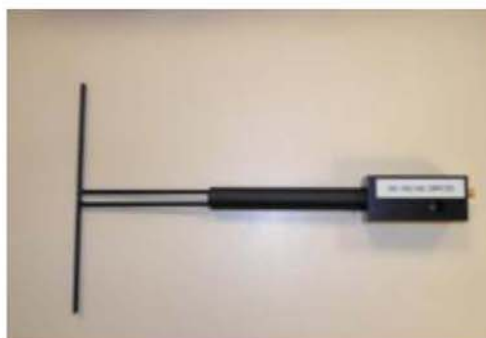
Figure 1 – Satimo COMOSAR Validation Dipole
