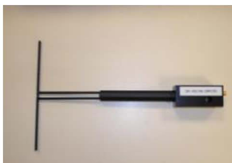
Figure 1 – Satimo COMOSAR Validation Dipole
