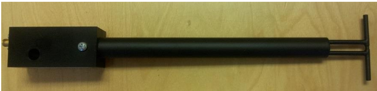
Figure 1 – MVG COMOSAR Validation Dipole
