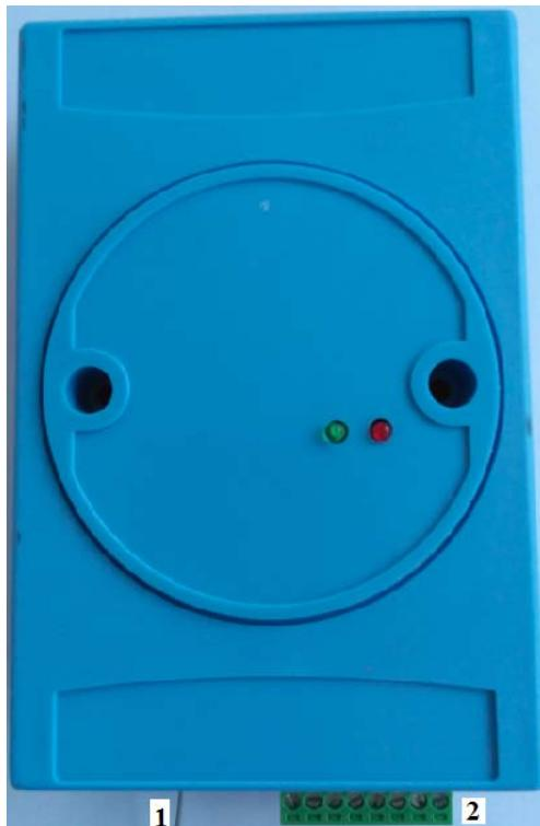
1、 external antenna 2、 power input terminal and GPRS expansion interface
