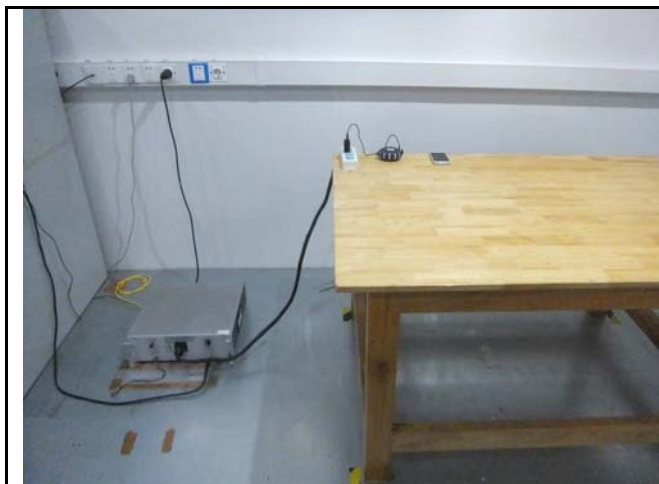
Conducted Emissions Test Setup Front View
