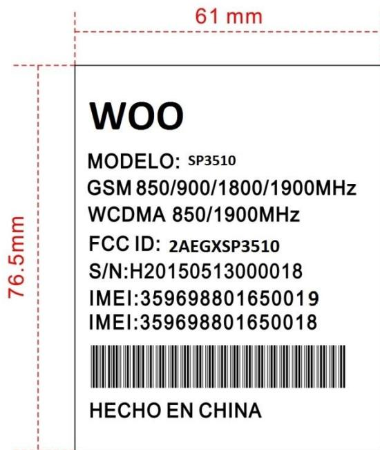
Label location: The battery is detachable so the label is visible to the users.
