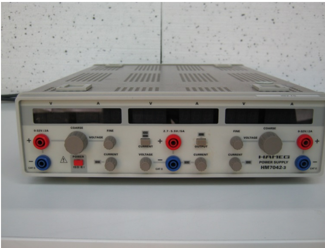
Photograph 2.3-1: Power supply HAMEG 7042-3
