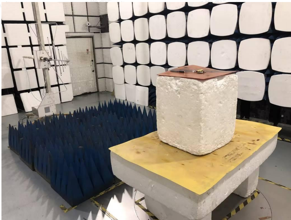
Radiated Emissions Measurement (Below 1GHz)
