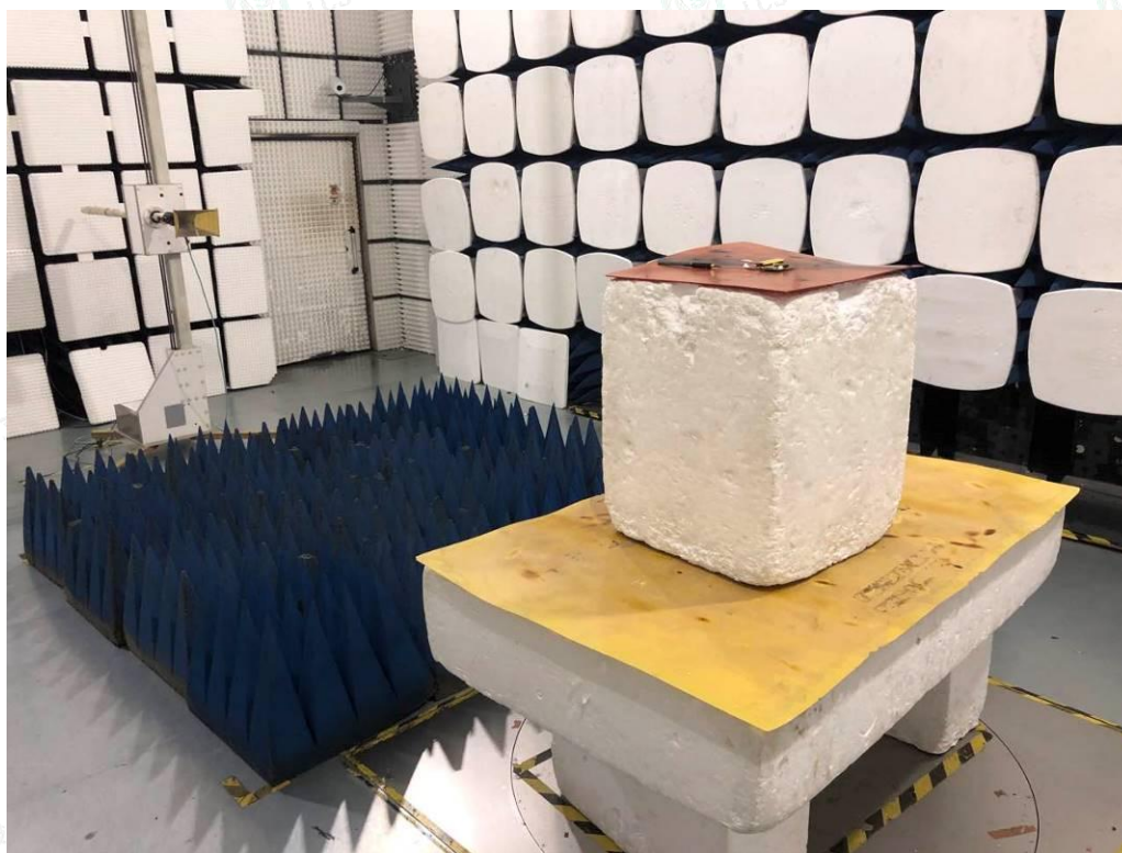
Radiated Emissions Measurement (Above 1GHz)
