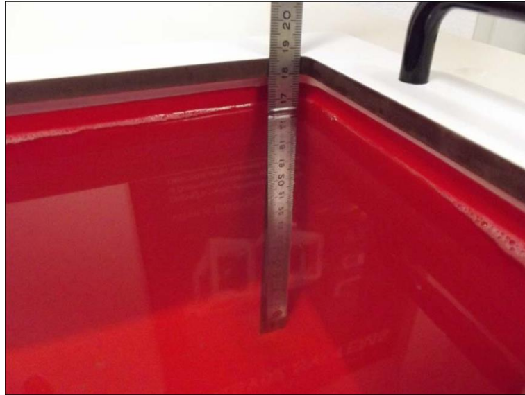
Photograph of the depth in the Body Phantom (900MHz)
